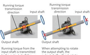
input shaft is transmitted to the output shaft for both forward and reverse rotational directions.
