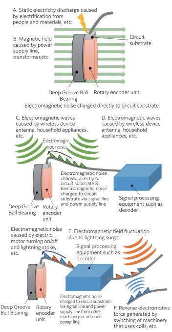
Fig. 12 Types of electromagnetic noise
