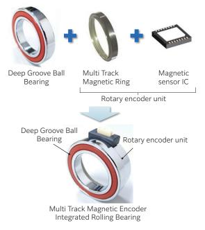
Fig. 2 Configuration of major components for the Multi Track Magnetic Encoder Integrated Rolling Bearing
