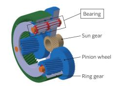
Fig. 4 Structure of co-axial type e-Axle planetary gear reducer
