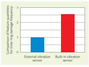
Fig. 8 Indentation bearing vibration verification test results
