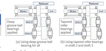
**Fig. 3** Example of rolling bearing arrangement in a simplified cross-sectional view of an e-Axle (motor and reduction gear)<sup>4)</sup>
