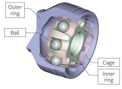
Fig. 9 Configuration of CFJ
