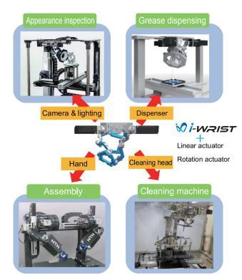
Fig. 2 Example of applications for i-WRIST<sup>™</sup>
