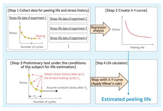
Fig. 1 Flow of the estimation method of peeling life<sup>4)</sup>
