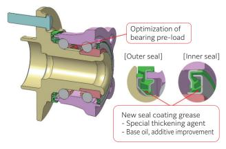
Fig. 5 Low Friction HUB Bearing  $\mathbb N$
