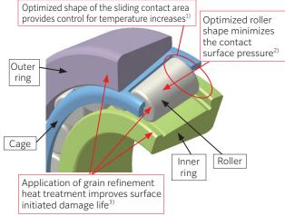
Fig. 2 Structure of ULTAGE Tapered Roller Bearing for Automotive Application
