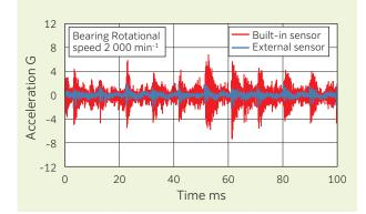
Fig. 12 Comparison of acceleration for built-in sensor and external sensor with abnormal bearing
