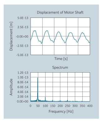
Fig. 23 Vibration analysis results of motor and shaft system<sup>23)</sup>
