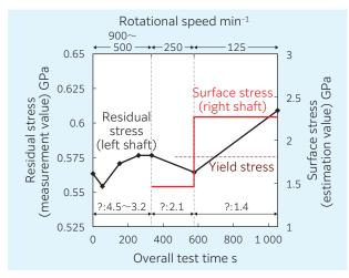
Fig. 4 Relationship between surface stress estimated by contact stress analysis and measured residual stress<sup>7</sup>
