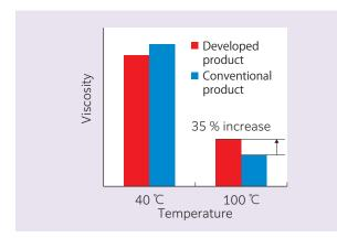
Fig. 12 Relationship between lubricating oil temperature and viscosity
