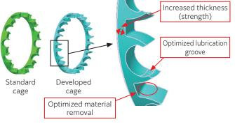
Fig. 1 Structure of developed cage
