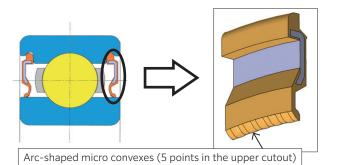
Fig. 4 Cross section of deep groove ball bearing with ultra-low friction seal<sup>5)</sup>
