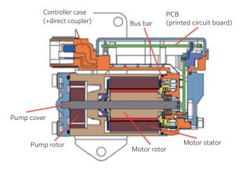
Fig. 9 Electric oil pump structure
