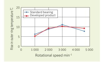
Fig. 16 Temperature increase characteristics for the developed product and standard bearing
