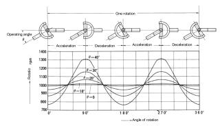
Fig. 3 Cardan Joint (cross shaft coupling)
