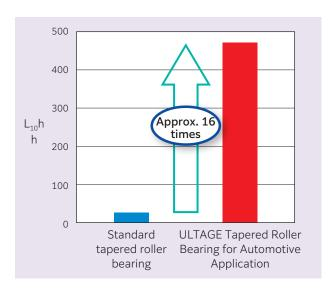
Fig. 21 Clean oil life test results for tapered roller bearings under high misalignment conditions<sup>15)</sup>
