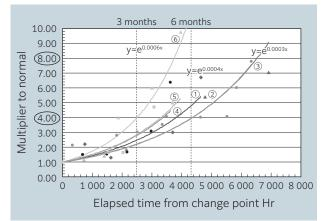
**Fig. 17** Bearing degradation curve at high frequency range acceleration<sup>19)</sup>
