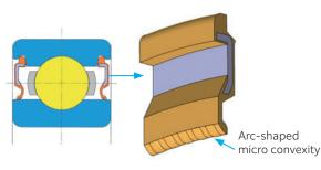
Fig. 1 Schematic drawing of developed seal
