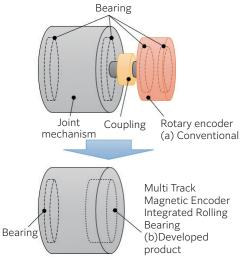
Using the developed product enables the rotary encoder to be integrated into the joint mechanism
