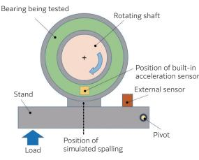
Fig. 8 Schematic drawing of testing equipment
