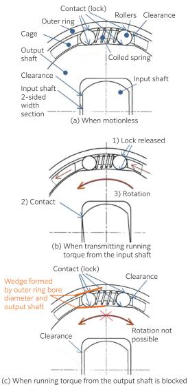
Fig. 3 TDL operating principle
