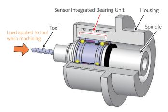
**Fig. 3** Example of application for the sensor integrated bearing unit on a machine tool spindle
