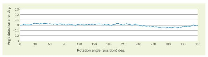
Fig. 11 Absolute angle detection error measurement results of Multi Track Magnetic Encoder Integrated Rolling Bearing
