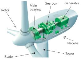
Fig. 10 Large wind turbine structure
