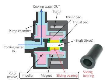
Fig. 4 Structure of electric water pump
