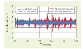
Fig. 11 Comparison of normal bearing and abnormal bearing built-in sensor output
