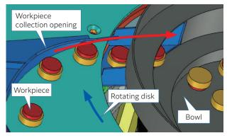
(b) Workpiece recovery Fig. 3 Workpiece separation and recovery
