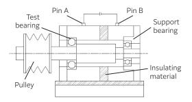
Fig. 13 Rolling life test machine
