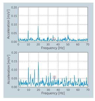
**Fig. 28** Envelope spectrum of acceleration signal (upper) before vibration, (lower) after vibration<sup>30)</sup>
