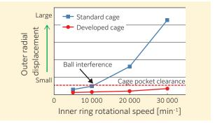
Fig.2 Difference in deformation due to centrifugal force (standard cage vs. developed "high speed" cage)
