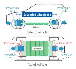
Fig. 2 Image of EV drive shaft arrangement
