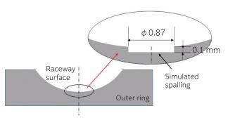
Fig. 9 Schematic drawing of simulated spalling
