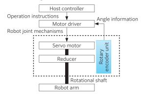
Fig. 4 Schematic drawing of positioning for robot joint mechanisms using the Multi Track Magnetic Encoder Integrated Rolling Bearing
