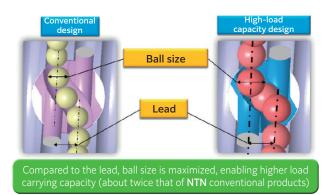
Fig. 7 Features of NTN ball screws
