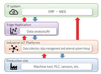
Fig. 1 Schematic drawing of industrial IoT platform
