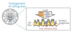
Fig. 2 Concept of load sharing theory
