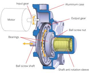
Fig. 8 Structure of the ball screw drive module for electronic hydraulic brake
