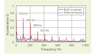
Fig. 13 Comparison of frequency analysis for built-in sensor and external sensor
