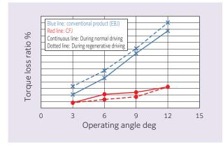
Fig. 13 Comparison of torque loss ratios
