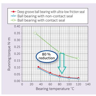
Fig. 6 Relationship between running torque and bearing temperature<sup>5)</sup>
