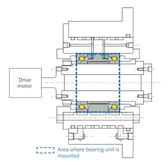
Fig. 5 Structure of evaluated spindle
