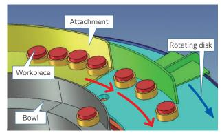
(a) Workpiece separation
