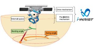
**Fig. 1** Schematic drawing of i-WRIST<sup>™</sup> unit
