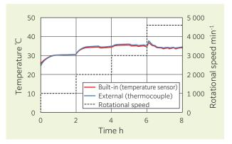
Fig. 14 Comparison of temperature taken with the built-in sensor and external thermocouple
