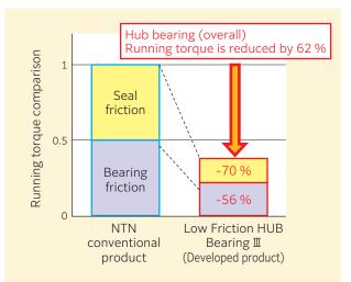
Fig. 2 Hub bearing running torque comparison (an example)
