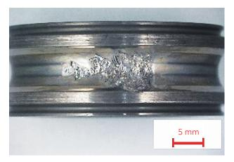
Fig. 10 Example of spalling damage
