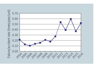
Fig. 9 Trends in wind turbine failure and accident  $\mbox{rates}^{17)}$
