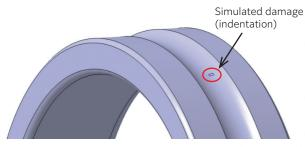
Fig. 7 3D illustration of the simulated damage (indentation) created on the bearing raceway surface
