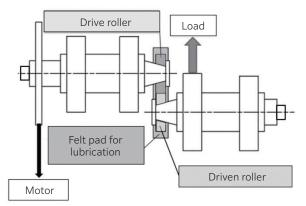
Fig. 5 Two-roller testing machine<sup>2)</sup>
