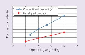
Fig. 15 Comparison of torque loss ratios
