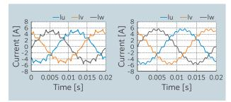
Fig. 24 Stator current (unsteady) (1DCAE and FEM)<sup>24)</sup>
