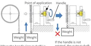
When the handle (input shaft) is rotated, the output shaft rotates and the weight rises.
