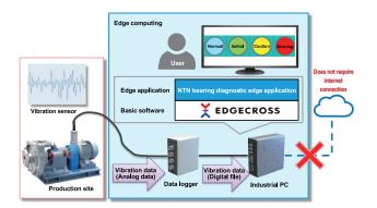
Fig. 8 Bearing diagnostic application
