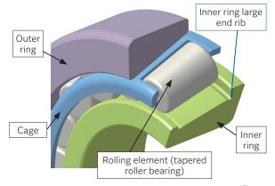
Fig. 14 Structure of tapered roller bearing<sup>15)</sup>
