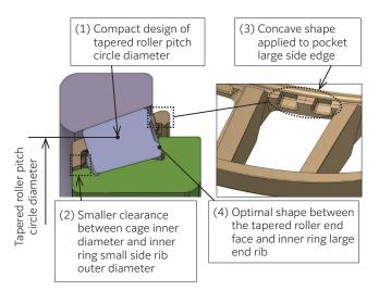
Fig. 16 Structure of "Low Temperature Rise and Low Torque Tapered Roller Bearing"<sup>16)</sup>
