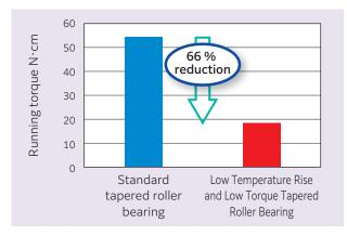
Fig. 17 Tapered roller bearing running torque test results<sup>16)</sup>
