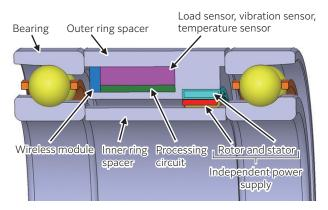
Fig. 2 Structural illustration of sensor integrated bearing unit
