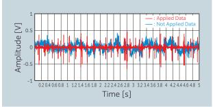
**Fig. 27** Time series data obtained by applying the proposed method and an anti-aliasing filter (low-pass filter with a cutoff frequency of 40 [kHz]) to the measured rotating noise of a bearing with outer ring failure<sup>29)</sup>
