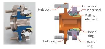
Fig. 4 GEN3 hub bearing
