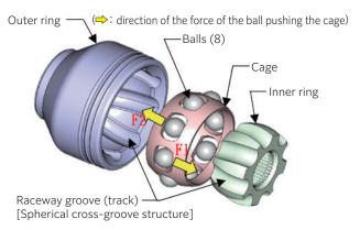
Fig. 6 CFJ structure and internal forces
