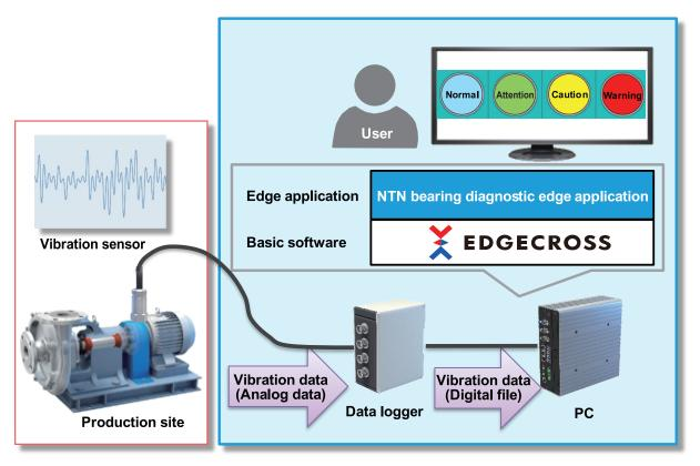
Fig. 2 Device configuration for bearing diagnostic application
