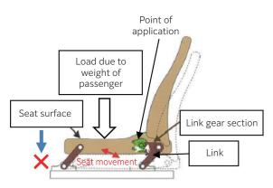
The torque diode prevents the link from falling over to maintain the seat position.
