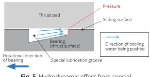
Fig. 5 Hydrodynamic effect from special lubrication grooves
