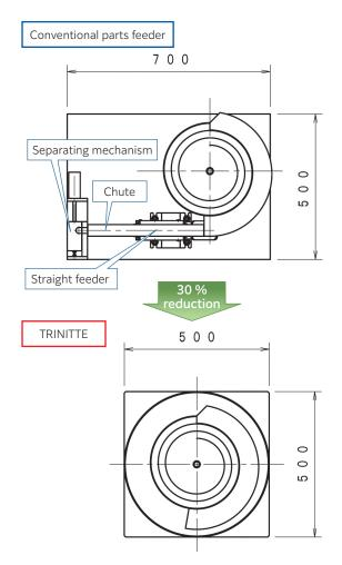
Fig.2 Comparison of size between conventional parts feeder and TRINITTE
