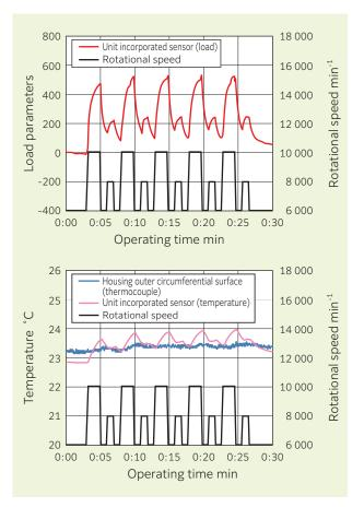
Fig. 6 Acceleration/deceleration test results
