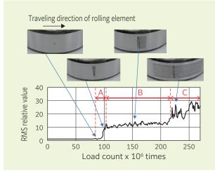
Fig. 1 Relationship between flaking progress and vibration acceleration<sup>8)</sup>
