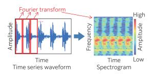
Fig. 3 Illustration of short time Fourier transform
