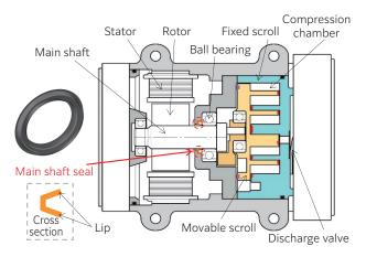
Fig. 1 Cross section of electric scroll compressors
