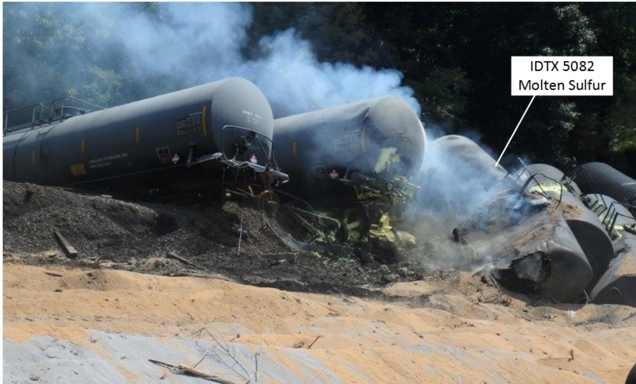
Figure 11. Burning molten sulfur released from tank car IDTX5082.
