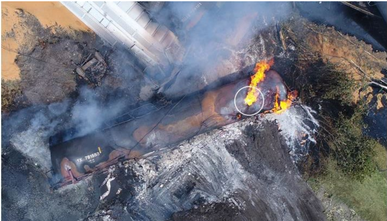
Figure 13. CBTX 781553 with puncture location circled, August 3, 2017, 2:46 p.m.
