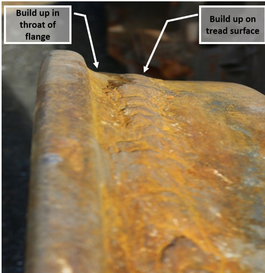
Figure 6. Closeup of wheel tread surface showing tread buildup on wheel of the 35th car.
