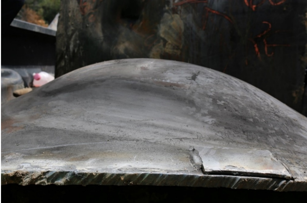
Figure 16. CBTX 781553 tank shell coupon showing bulge profile, August 5, 2017.
