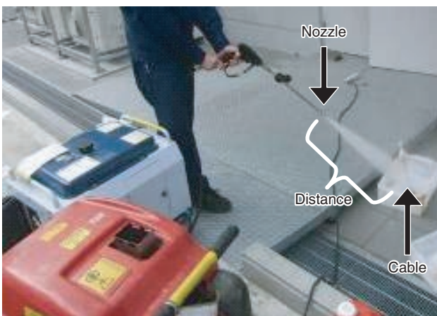
Fig. 5. Damage-reproduction experiment using a high-pressure water sprayer.
