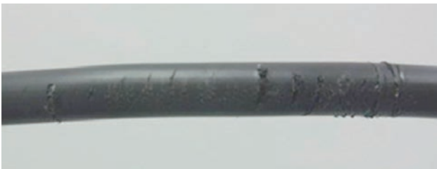
Fig. 4. Cable damaged by a sharp-edged object.
