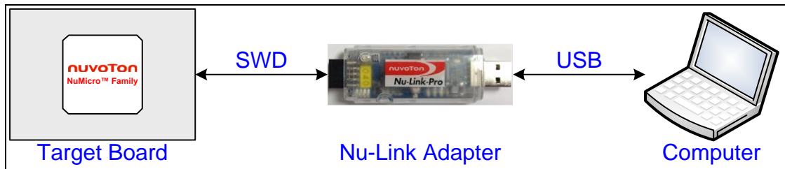
Figure 4-1 Nu-Link Adapter Connection Diagram
