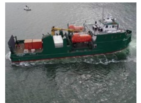
M/V Manu'atele, undergoing sea trials. Two 850-hp Caterpillar C32 ACERT Tier 3 engines pull the ferry in full reverse. A nearby 25-foot sailboat gives a sense of scale.
