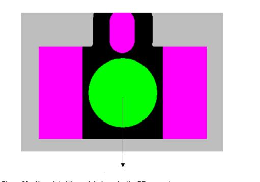
• We recommend to place a non-plated through hole under the RF connector to minimize the insertion loss as shown in <u>Figure 26</u>.
