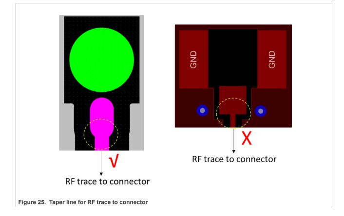
• RF trace to RF connector pad transition must be tapered to avoid discontinuity and high insertion loss, especially at 5 GHz band. An example is shown in Figure 25.
