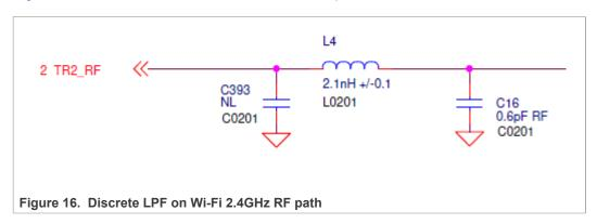
Figure 16 shows the filter circuit for Wi-Fi 2.4 GHz path.
