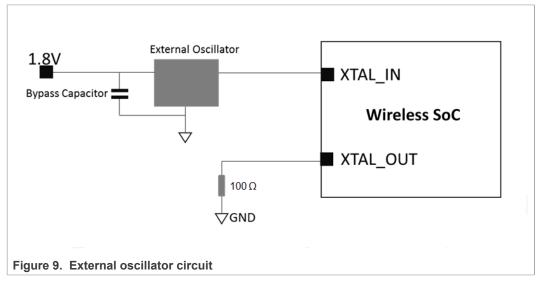
An external 26 MHz external oscillator may be used as reference clock source. If using an external oscillator, make sure its frequency accuracy meets the ±20 ppm IEEE specification over the operating temperature range of the product. Refer to IW416 data sheet for the oscillator requirement specification.
