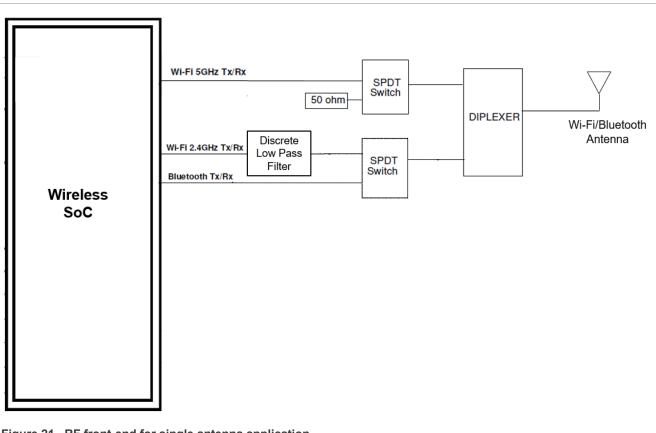
Figure 21. RF front-end for single antenna application
