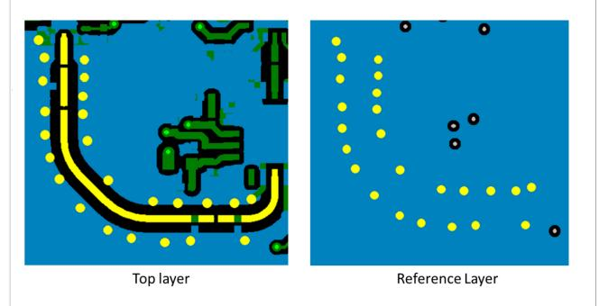
• Place stitching vias between the top and reference ground layers to increase isolation as shown in Figure 23.
