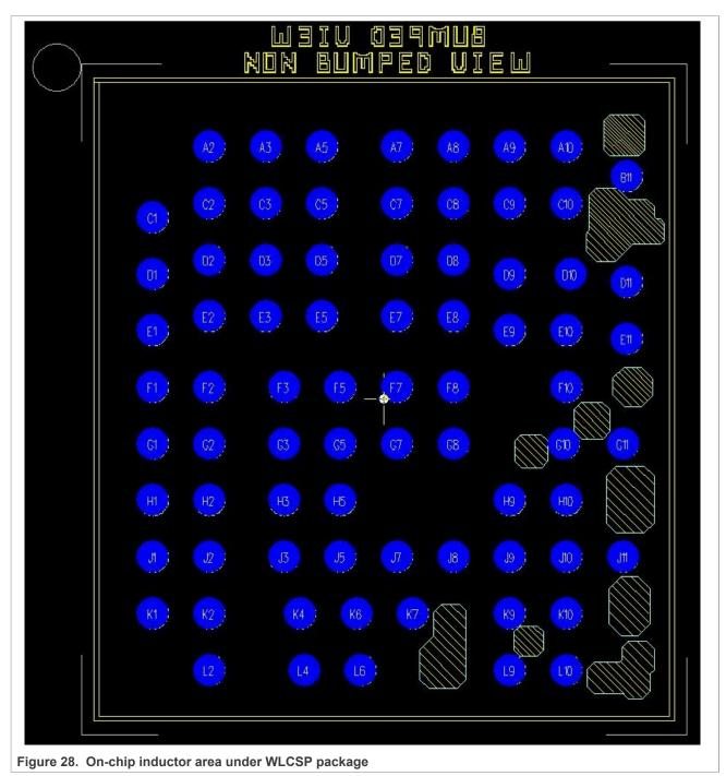
For additional details, refer to DXF drawing layer included in Wireless SoC WLCSP reference design PCB layout file on NXP website.
