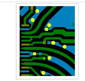
Figure 24. Ground pour along with RF trace end with a ground via
