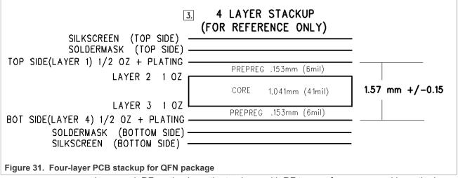
In general, RF routing is on the top layer with RF trace reference ground is on the layer 2
