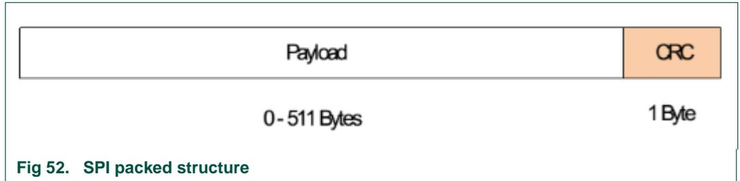
Fig 52. SPI packed structure
