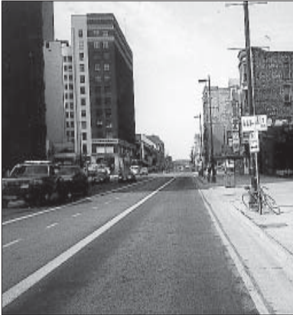
Bi-directional contra-flow bicycle lane on Hennepin Avenue between 4th and 5th Streets, looking south.
