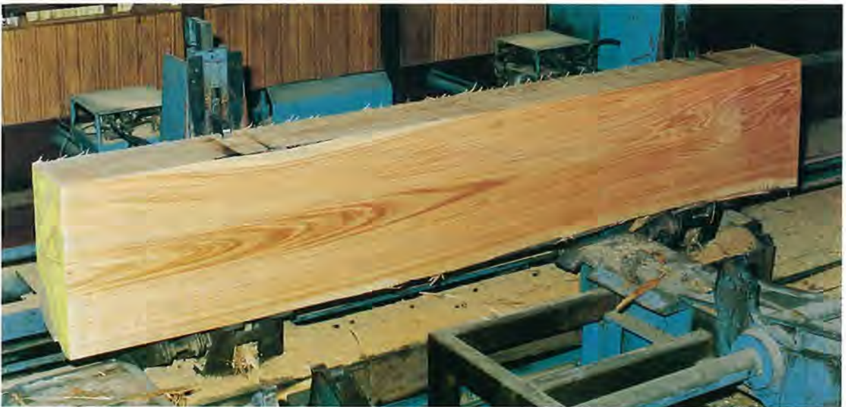
Fig. 17 - Bandsawing 53-year-old Cupressus macrocarpa .
