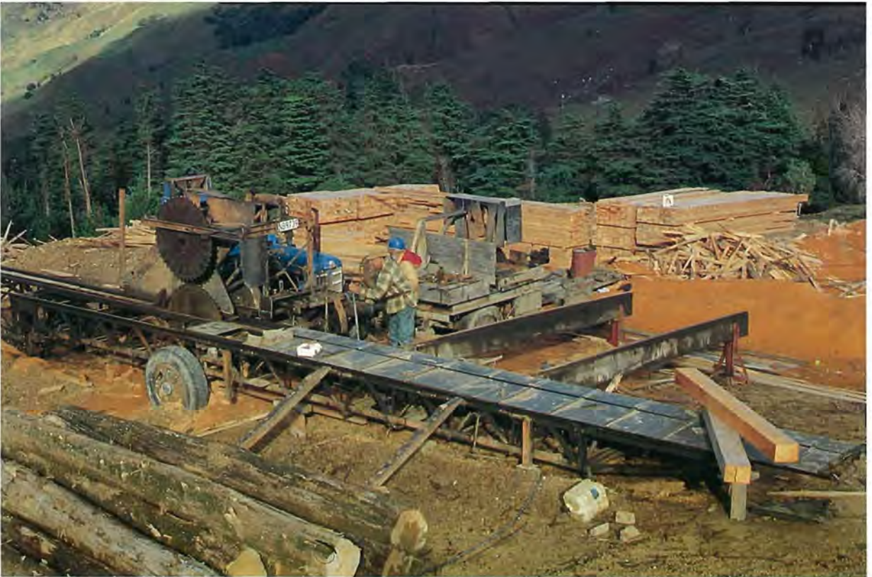
Fig.19 – Sawing Cupressus macrocarpa (from stand in background), Te Puia Springs, East Cape.
