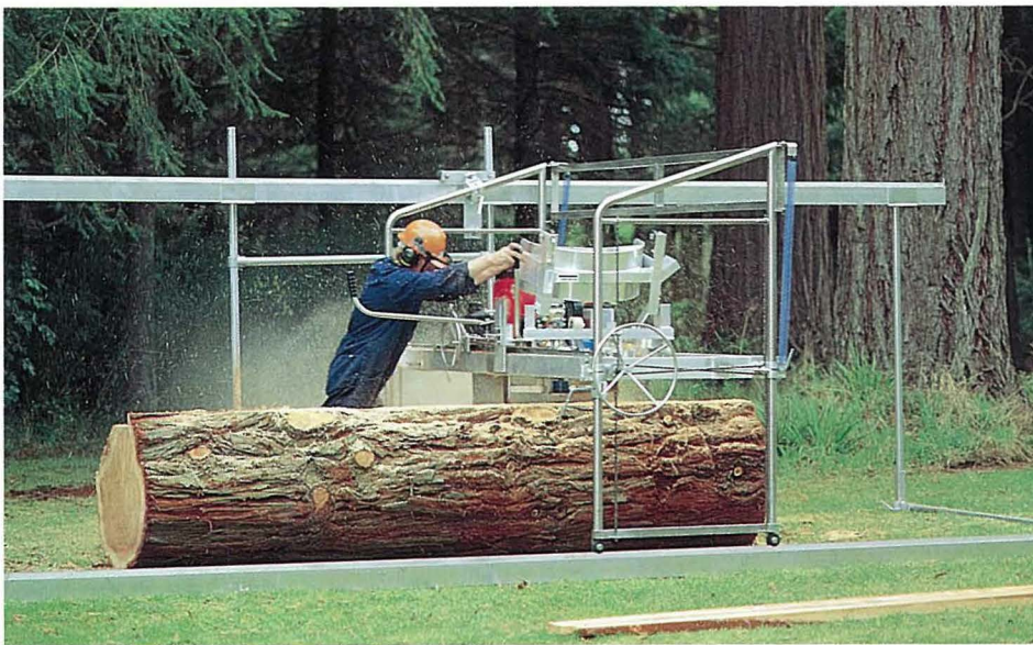
Fig. 13 – Converting large coast redwood log on site using portable sawmill.
