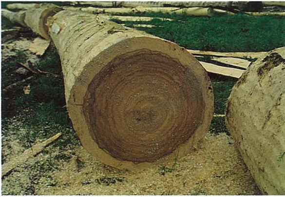
Fig. 29 - 'Blackheart', the zone of bacterial infection, also known as 'bacterial wetwood', is clearly evident in this P. deltooides × P. nigra 'I 214' log.
