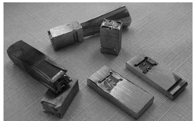
Fig. 1 The process of making metal type. From left to right: a steel punch, a copper strike, and a justified matrix of a decorative capital A. At the back: a cast type with its jet still attached, and a cast type dressed to form the finished sort at type height.
