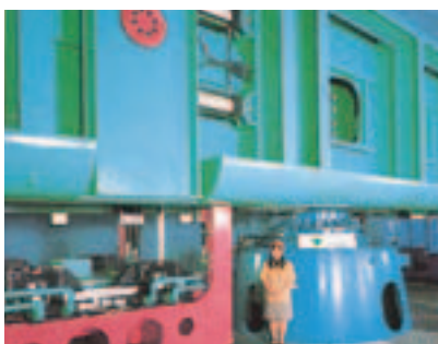
Geotechnical Centrifuge System Experimentally simulates ground movement using a scale model
