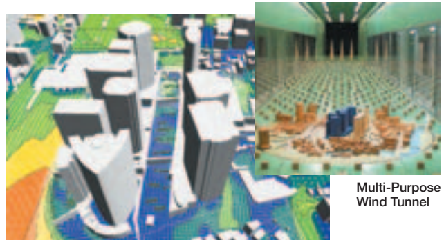
Numerical Simulator for Wind Environment Predicts wind environments around a building complex
