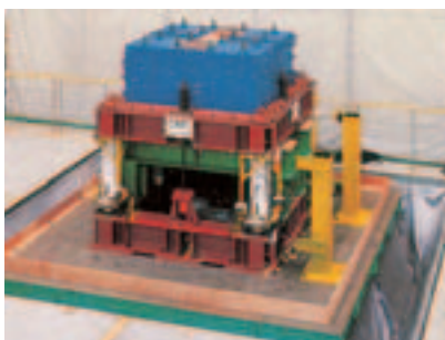
Tri-axial Shaking Table Capable of simulating earthquakes twice the magnitude of the 1995 Kobe Earthquake
