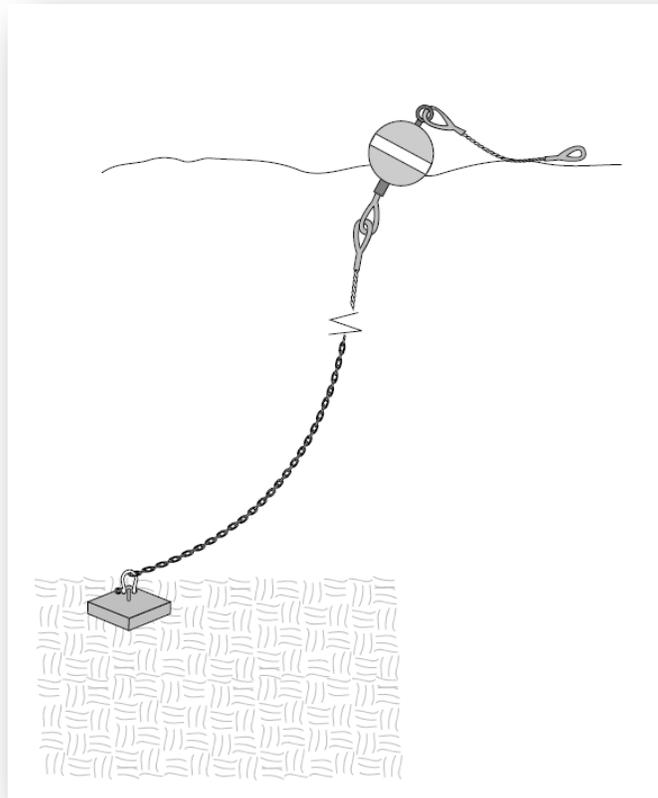
Figure 77. Traditional mooring buoy system (Project AWARE Foundation, 1996).
