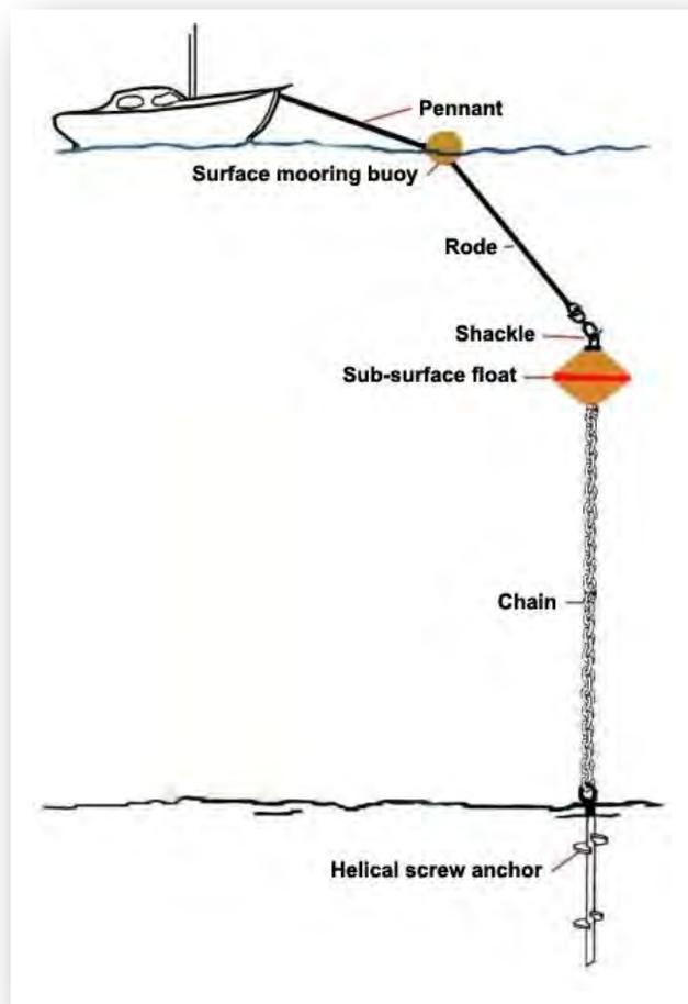
Figure 79. Example of a helical screw anchor system.
