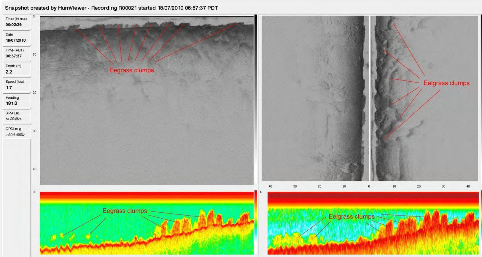
Figure 43. An example of raw side scan sonar data as viewed by the HumViewer software.
