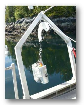
Figure 6. Towed video camera system about to be deployed.
