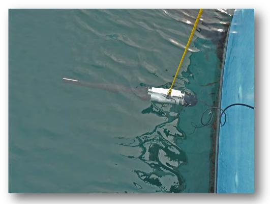
Figure 12. Side scan sonar towfish in towing position.
