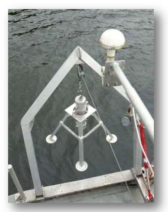
Figure 10. High definition drop camera in the lander frame.
