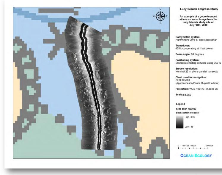
Figure 44. An example of a georeferenced side scan sonar image from the Lucy Islands study site on July 18<sup>th</sup>, 2010.
