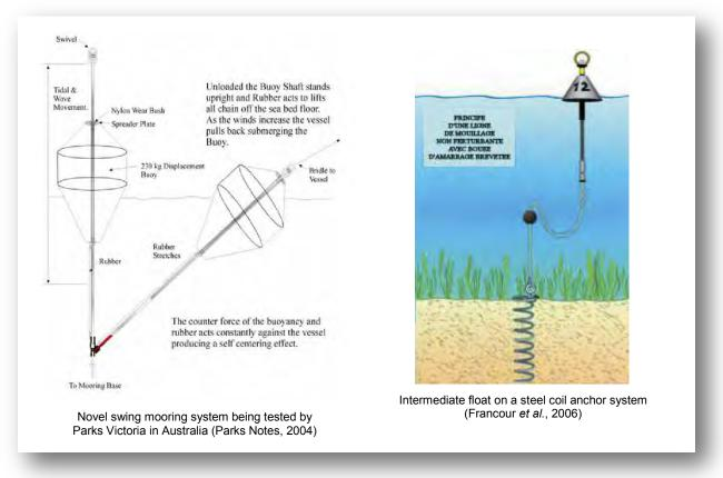
Figure 81. Examples of mooring systems which prevent the mooring chain from dragging through the benthos.
