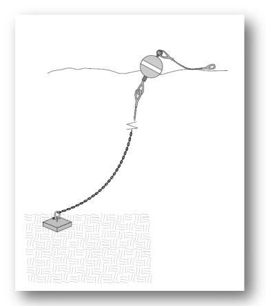
Figure 77. Traditional mooring buoy system (Project AWARE Foundation, 1996).
