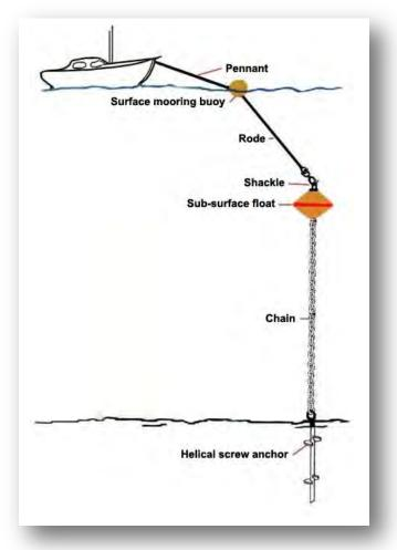
Figure 79. Example of a helical screw anchor system.
