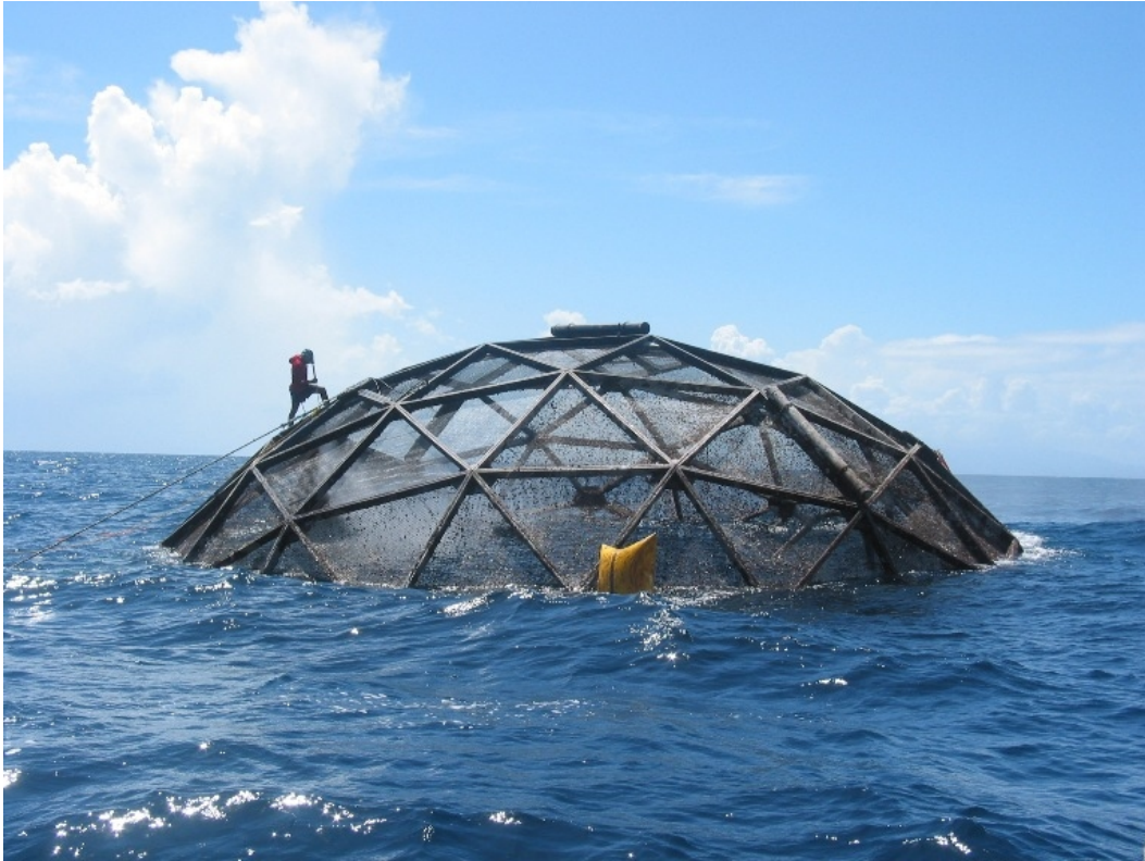
Figure 4.18. Floating “AquaPod” steel-and-wire mesh net pen for Snapperfarm, Inc. to raise cobia in deep water off Culebra, Puerto Rico (source: http://gcaptain.com/maritime/blog/wp-content/uploads/2009/03/aquapod_fish-farm1.jpg ) (accessed March 21, 2010).
