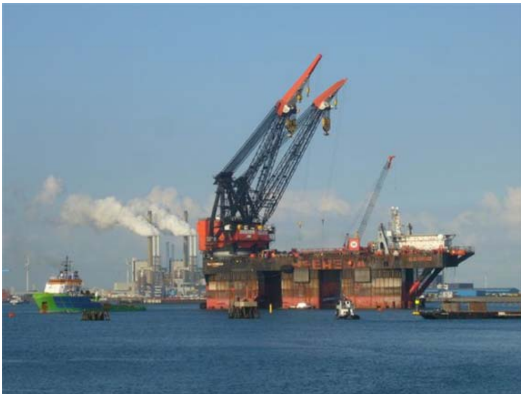
Figure ES.4. The Heavy Lift Vessel Hermod is in the 4000 ton lift category that would be required to decommission the larger California platforms (source: Scheepvaartnieuws, scheepvaartnieuws.punt.nl/upload/mot_1496.jpg , accessed January 28, 2010).
