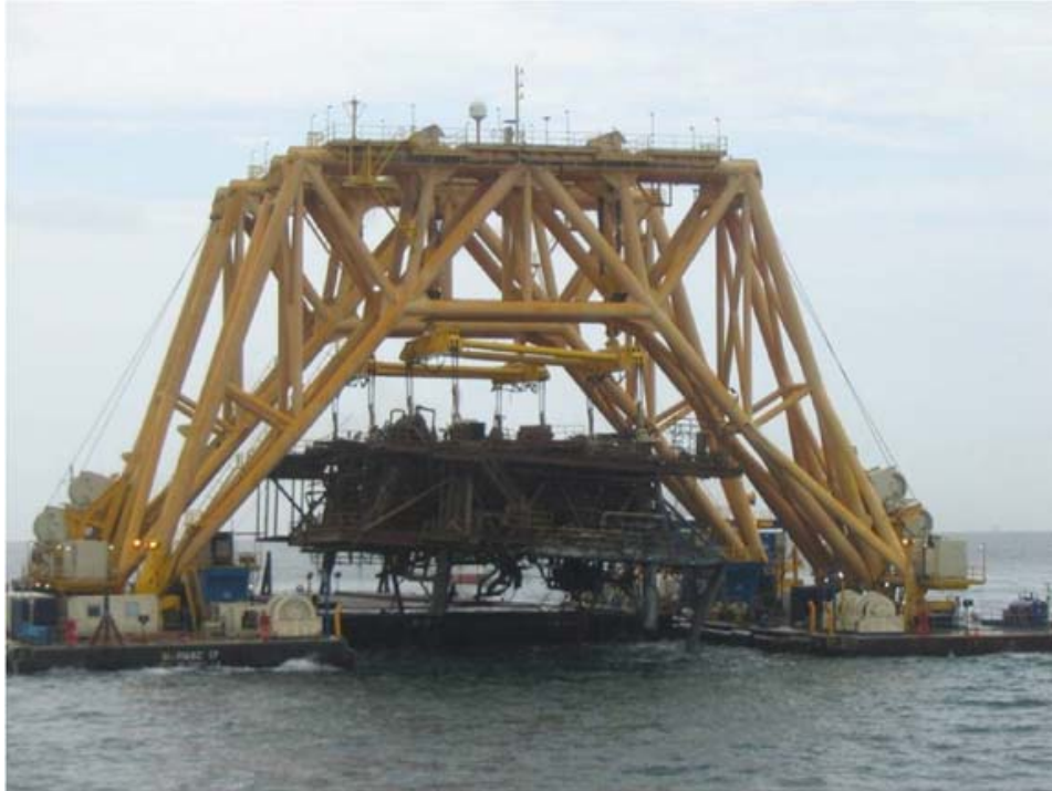
Figure 4.4. Bottom feeder lifting device (image courtesy of Proserv Offshore, Inc.).
