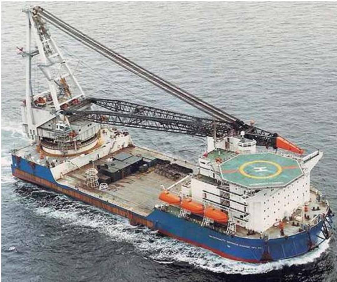
Figure 4.5. The McDermott DB50 is one of several derrick barges that fall into the 4000 ton class of HLVs (source: technology, http://www.offshore-technology.com/projects/north-america_gallery.html , accessed January 28, 2010).
