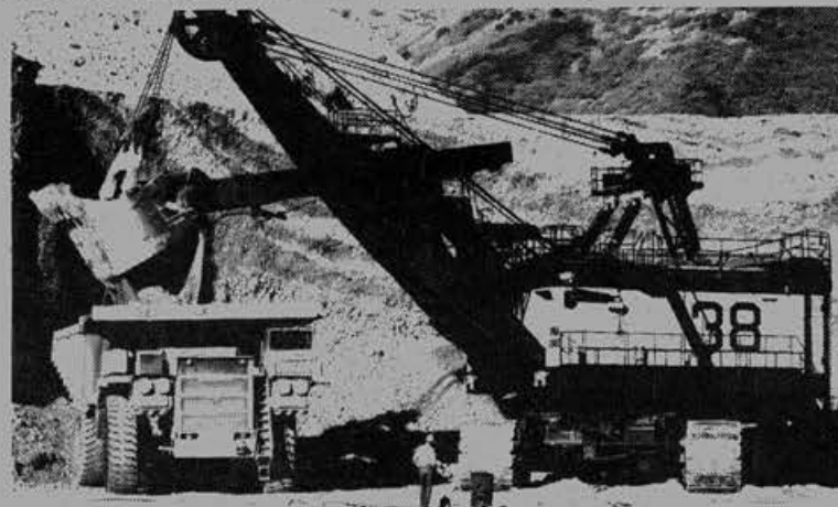
KENNECOTT COPPER CORPORATION'S new 25-cubic-yard electric shovel is put into operation in the upper west side area of the Utah copper mine. The first of four giant shovels ordered, it is believed to be the largest of its kind in the nonferrous mining industry. (Photo by Kennecott Copper Corp.)
