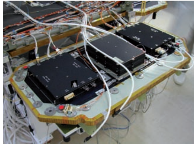
Fig. 3: BEX processors onboard the CoRoT space telescope.
