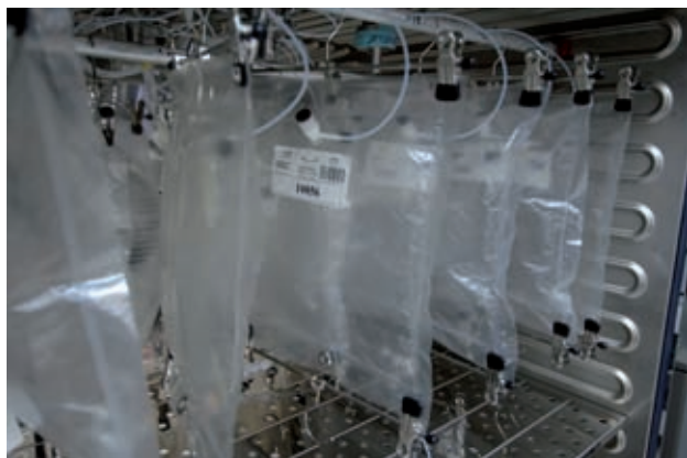
Fig. 2: tedlar bags ready for automatic proton transfer reaction mass spectrometric analysis
