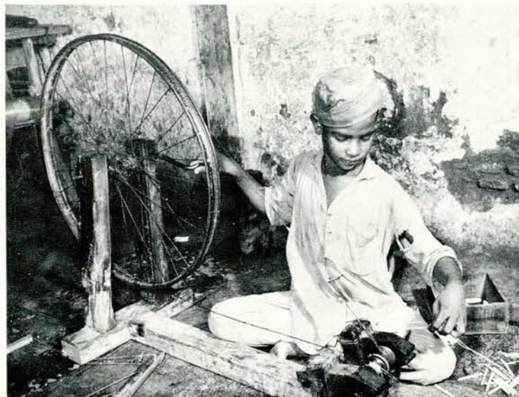
A young boy prepares spools of thread for home weaving on a spinning wheel built from an old bicycle.
