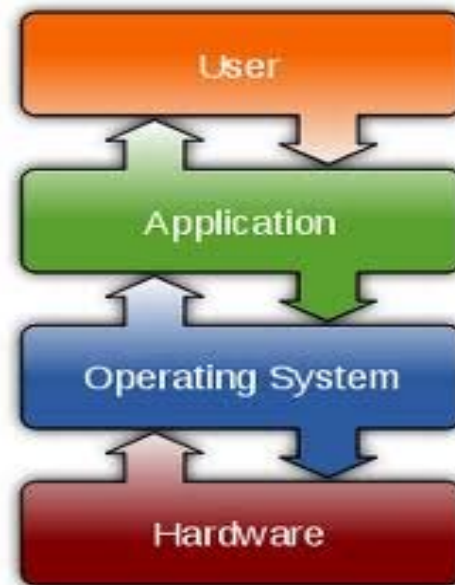
Figure 5: Diagram showing how operating system controls hardware, application programs and indirectly, users
