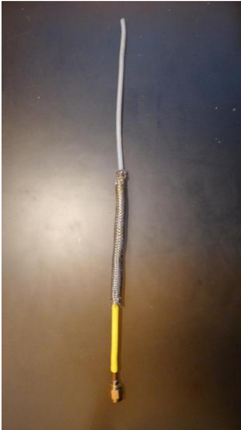
Figure A4: The test antenna
