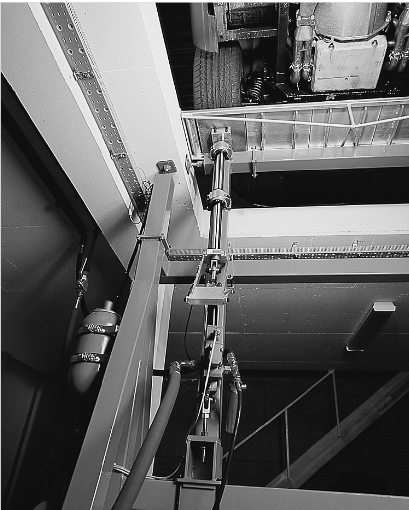
The Ohlins four poster rig can reproduce both dynamic and aerodynamic forces and is widely used by race teams and car manufactures.
