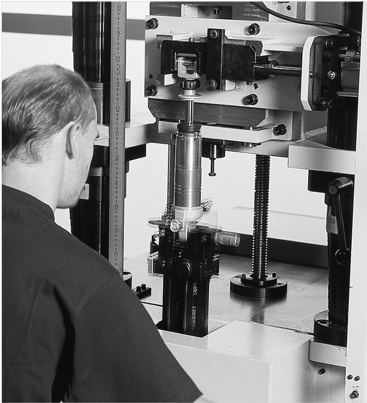
All Öhlins dampers, not just the racing dampers, are dyno tested before they are delivered to the customer.
