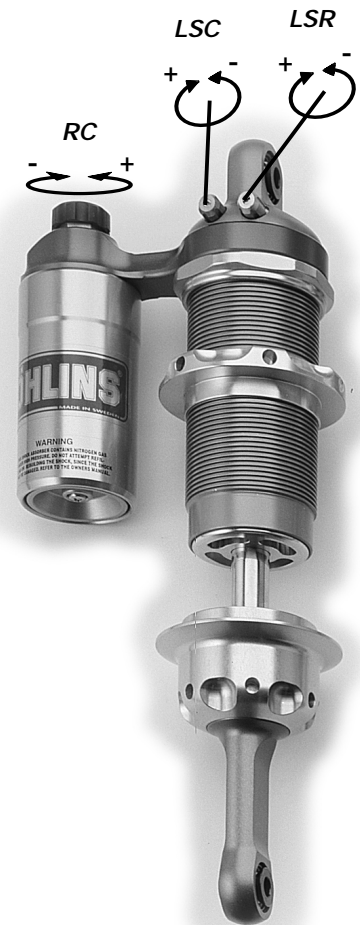
Figure 6. Standard external adjusters. - = soft. + = hard.
