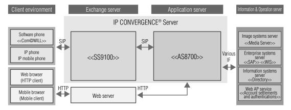
Fig. 1 Configuration of the SS9100/AS8700
