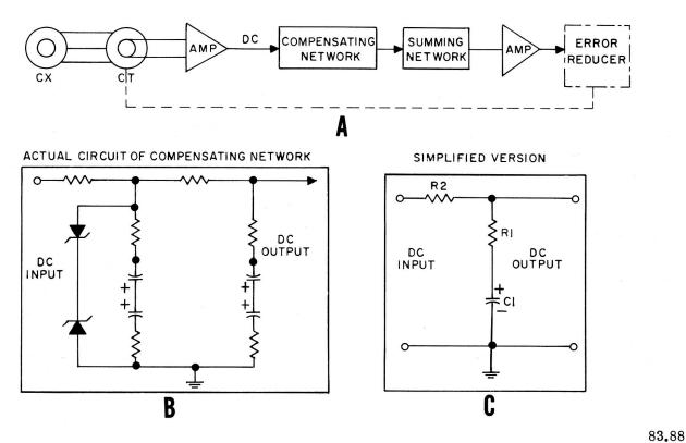
Figure 7-23. — Integral control: A. Simplified block diagram of power drive servo; B. Integral control circuit of compensating network; C. Simplified circuit of compensating network.
