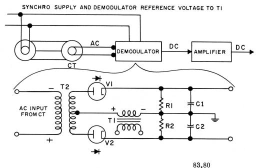
Figure 7-13. — Diode vacuum tube demodulators.
