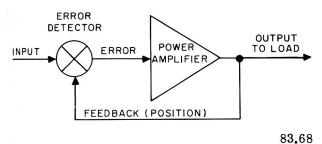
Figure 7-1. — Elementary servo in its simplest form: block diagram.
