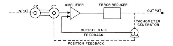
A VELOCITY FEEDBACK USING A TACHOMETER
