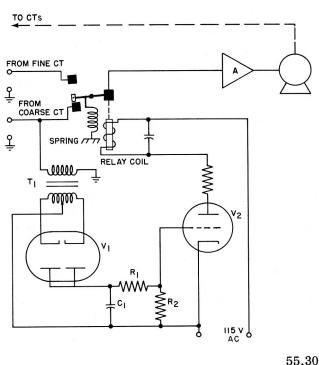
Figure 7-9.—Relay synchro changeover circuit.
