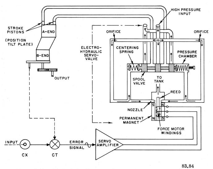
Figure 7-19. — Electrohydraulic servovalve operating in a control system.
