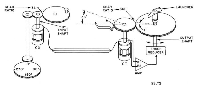
Figure 7-6. — Launcher power drive using a fine synchro system.
