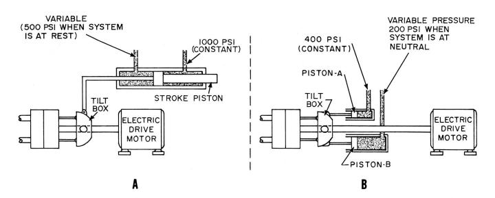
Figure 7-18.—Putting tilt on the A-end: A. Pressure on one piston; B. Pressure applied to two pistons. 83.83
