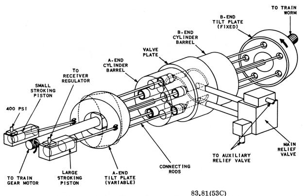
Figure 7-14. — (combination A-end and B-end).
