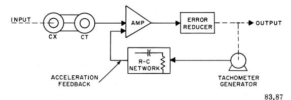
Figure 7-22. — Reducing hunting and overshooting: Acceleration feedback.
