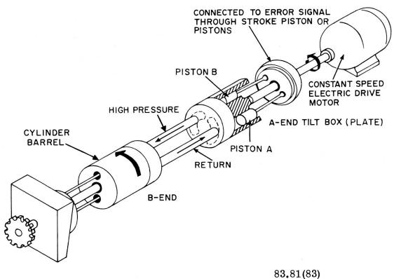
Figure 7-16. — A-end and B-end operation.
