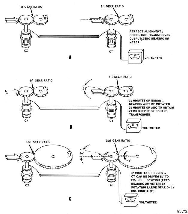
Figure 7-5. — Electrical error in a synchro system: A. A perfect synchro transmitter connected to a perfect control transformer; B. Synchro transmitter and control transformer each with electrical error of 18 minutes; C. "Fine" synchro system using 36:1 gear ratio to reduce error.
