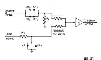
Figure 7-10. — Semiconductor diode synchro changeover network.
