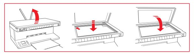
2 Place the original document or photo to be scanned face down on the scanner glass and aligned with the upper left corner. Close the top cover.
