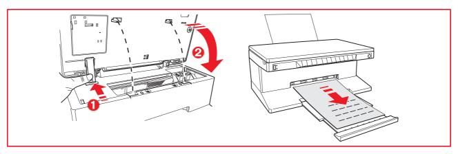
If a new cartridge is installed, the printer will automatically perform a cartridge recognition procedure which lasts at least 3 minutes. An ink cartridge alignment page will then be printed to indicate that the newly installed ink cartridge was automatically aligned. For information see "Aligning the Ink Cartridges".
