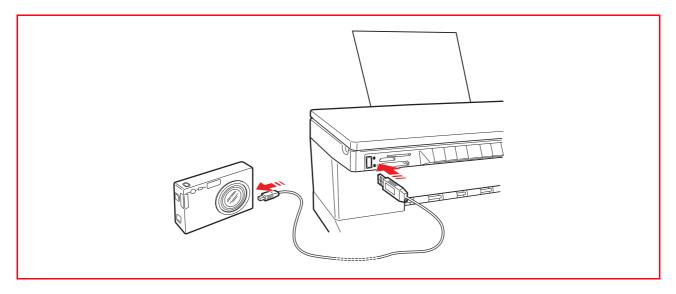
The USB status LED illuminates to indicate that a digital camera is connected.
