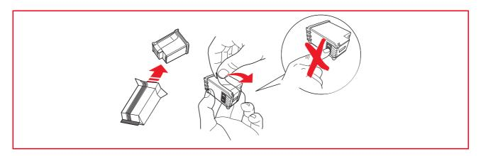
Hold the ink cartridge with its nozzles facing downward and contacts facing the rear of the printer, and insert the colour cartridge in the left carrier and the black or photo cartridge in the right carrier.
