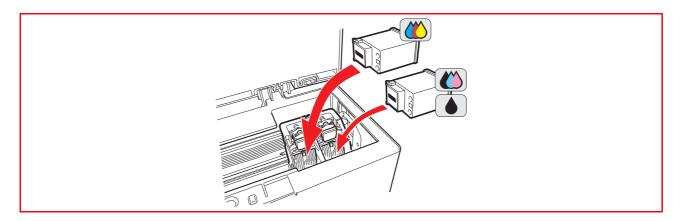
8 Push the ink cartridge firmly inward until it is locked by the securing clip.
