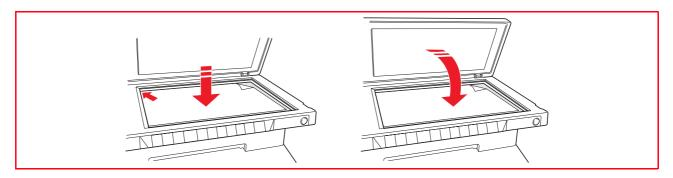
If the top cover was removed, replace it after copying by sliding its tabs into the related slots on the rear of the printer until they click into place. Close the top cover.
