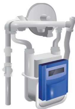
Gas meter installed with a seismic sensor
