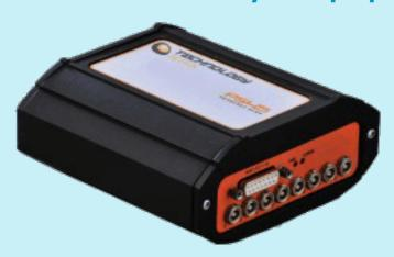
The Ethernet connection simplifies the link between laptop and Pocket-Scan and eliminates the need for a PCMCIA type II card slot. The Ethernet system requires minimal initial setup with no special drivers and will communicate with any Ethernet enabled PC.
