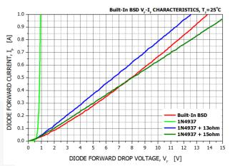
Figure 41. V-I characteristics of Bootstrap Diode in SPM3 V5 products
