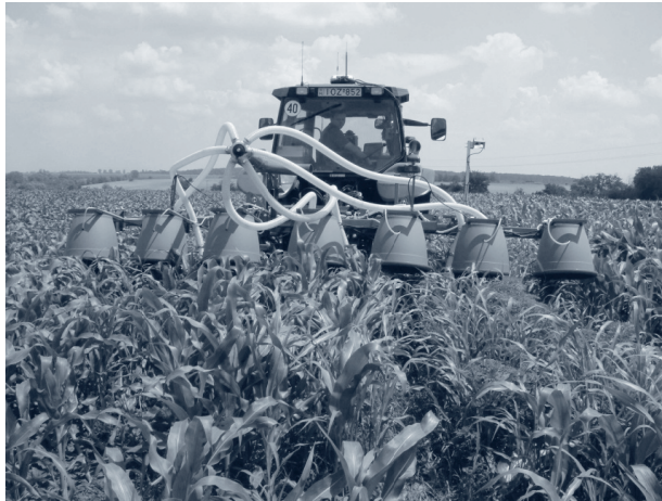
Fig. 2 WeedSeeker sensor-sprayers shielded by plastic container.
