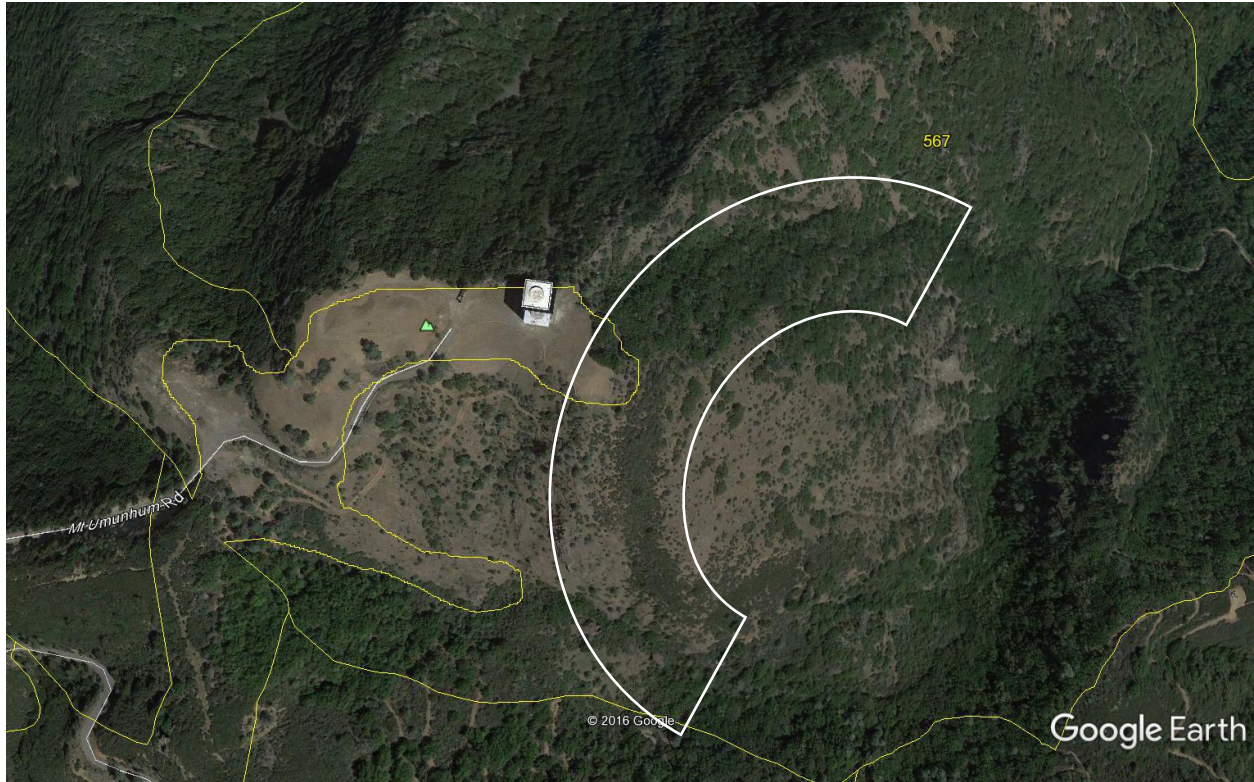
Figure 7.7.2. A potential example of the effect of aspect on vegetation growth. The curved band could be explained by an upturned layer of more easily weathered rock is tilted downward to the east and is exposed on the south and north sides of this ridge. These geological strata are visible elsewhere in the local area. The south slope half can be expected to be hotter and drier and less soil formation through centuries of time. The north-facing slope could be expected to be cooler and retain more moisture after rains. It would therefore develop more vegetation inputs and a deeper soil. Sampling of this band should show weaker sedimentary rocks such as shales and weakly cemented sandstones. This has not been confirmed in the field.
