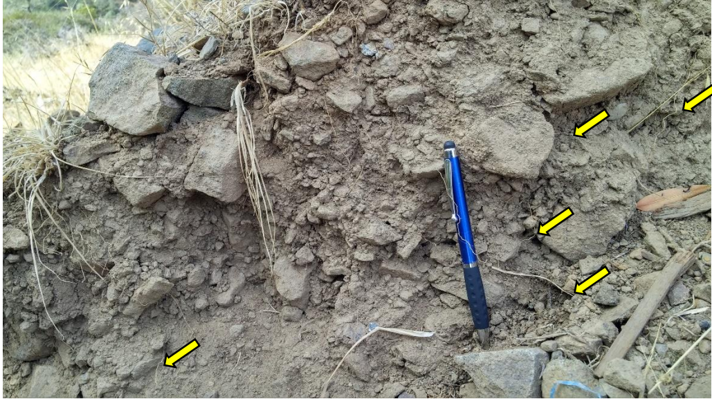
Figure 1: Detail photograph of soils on summit. Note the occurrence of small spaces between gravels and roots extending several feet into the soil (arrows)
