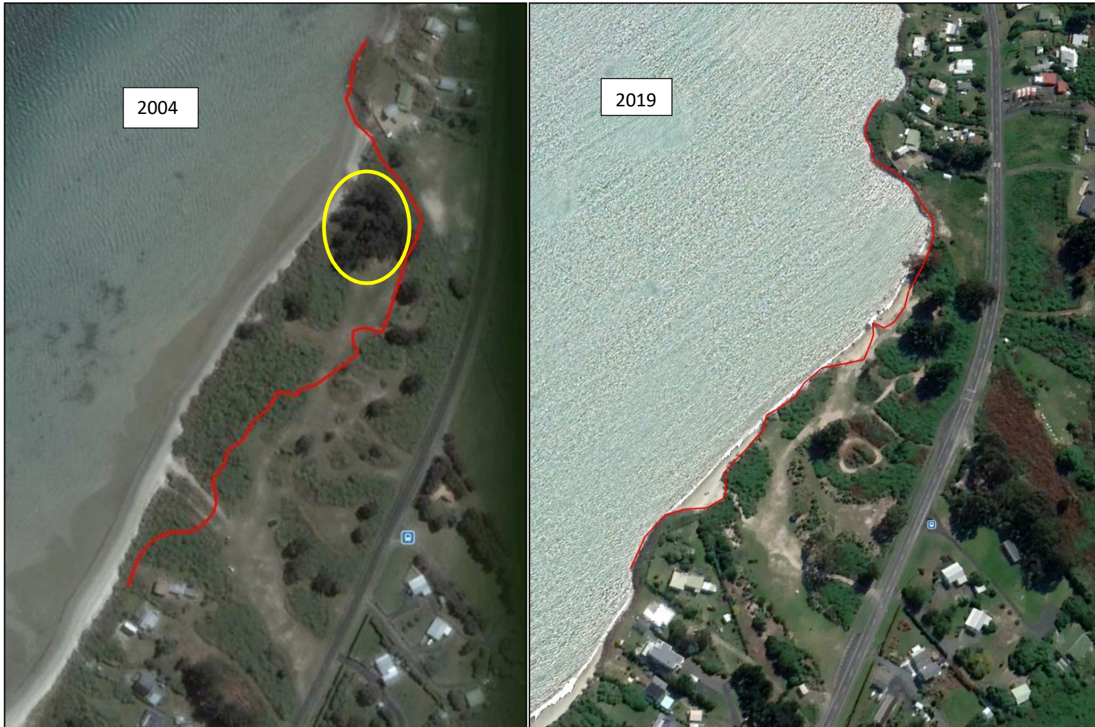
Figure 2: Aerial photographs from Google Earth of the northern end of Te Rauone beach showing the extent of vegetation in 2004 (left photograph) compared with the same stretch of beach in 2019 (right photograph). The red line indicates the approximate position of the mean high-water springs line in 2019 that has moved inland up to c. 65 m. Some of the large trees over the northern part of the reserve (yellow circle) that are now only stumps on the beach/foreshore.
