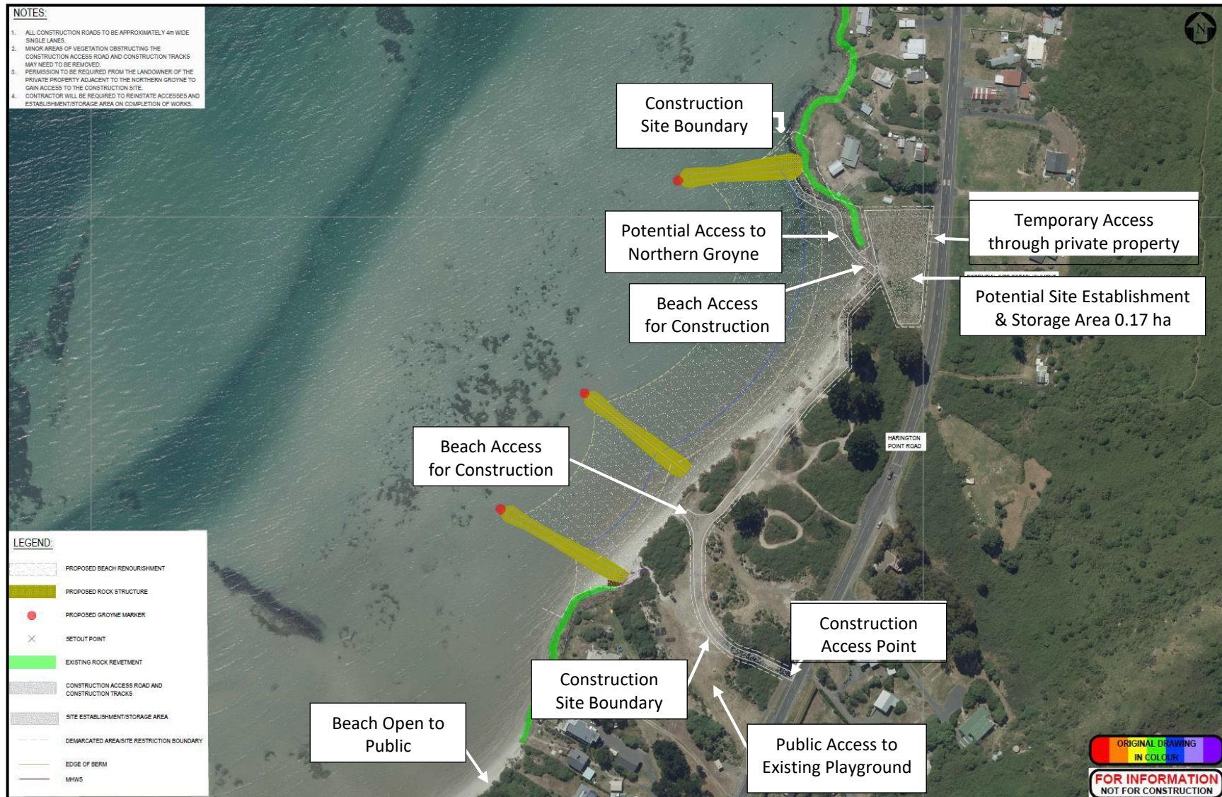
Figure 3: Aerial photograph showing the site plan for the scheme including public and construction access tracks along with a 0.17 ha site establishment area on private land over the northern part of the site. Image supplied by BECA.
