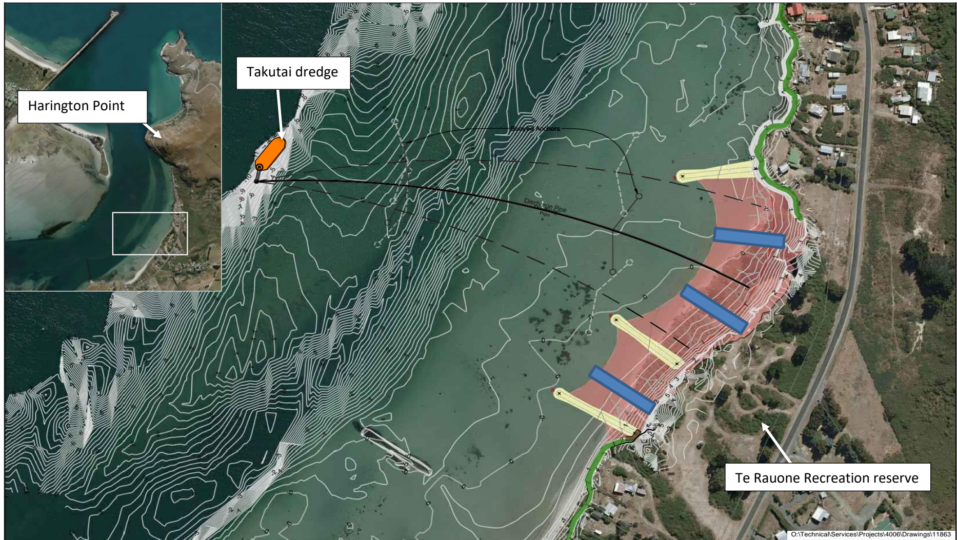
Figure 1: Site location of the Te Rauone Beach nourishment scheme showing footprint (pink shading) and location of the proposed groynes (cream shaded areas projecting into the harbour from the beach). Indicative locations of impact transects, that were surveyed for benthic fauna and flora, are shown in blue (see Figures 5 and 6 below for a detailed sampling map. Base photo supplied by Port Otago Ltd. The proposed location of the backhoe dredge, Takutai, that will pump sediment onshore is also shown.
