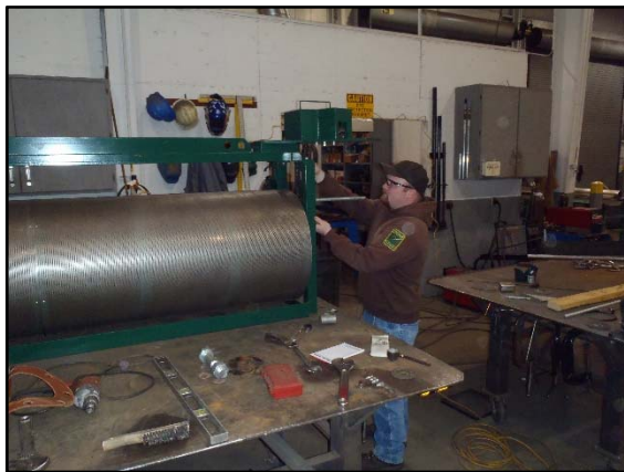
Technicians service many screens onsite, but larger repairs are completed at the screen shop.
