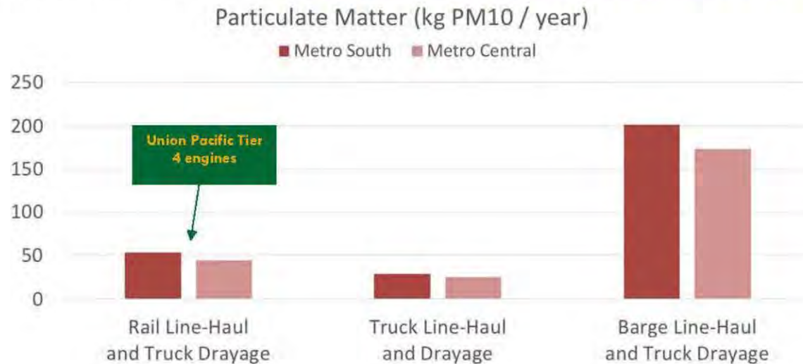
Figure 4: WM Approach direct PM 10 from waste transport modes (based on WM data and assumptions) for Metro Central and South County Transfer Stations. NOTE: Smaller bars are preferable (i.e. fewer annual emissions)
