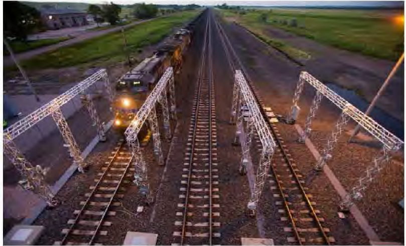
Remote rail car inspectors receive detailed images of rail cars as they travel through Machine Vision.
