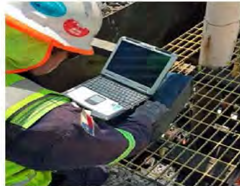
Guided wave technology allows Union Pacific's fuel team to take a closer look at the railroad's underground assets.
