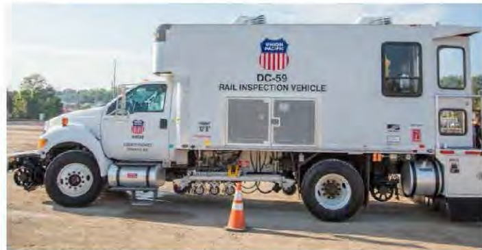
The rail test truck's 48 ultrasonic transducers identify air gaps in the track, indicating the rail part needing maintenance, with high-frequency sound.
