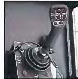
Joystick control with individual fingertip hydraulic and electronic controls for smooth precise control
