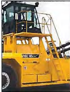
Anti-slip steps and handrails for 3-point mounting and dismounting (meets new proposed ANSI B56.1 standard)
