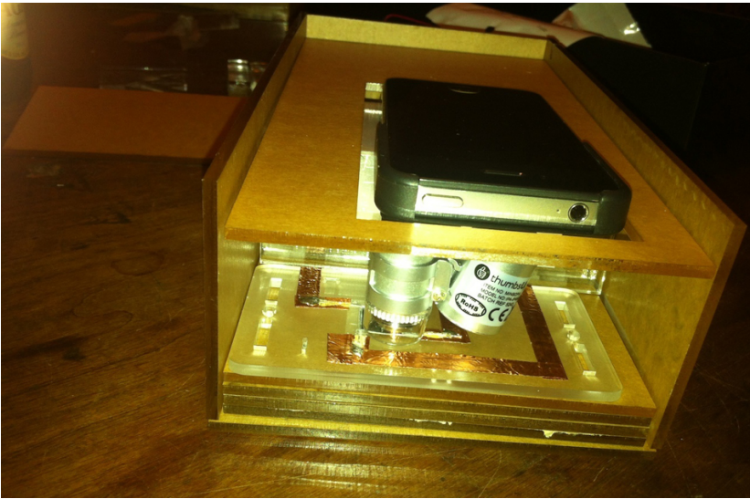
Figure 9-1. iPhone with microscope attachment positioned above parametia stage
