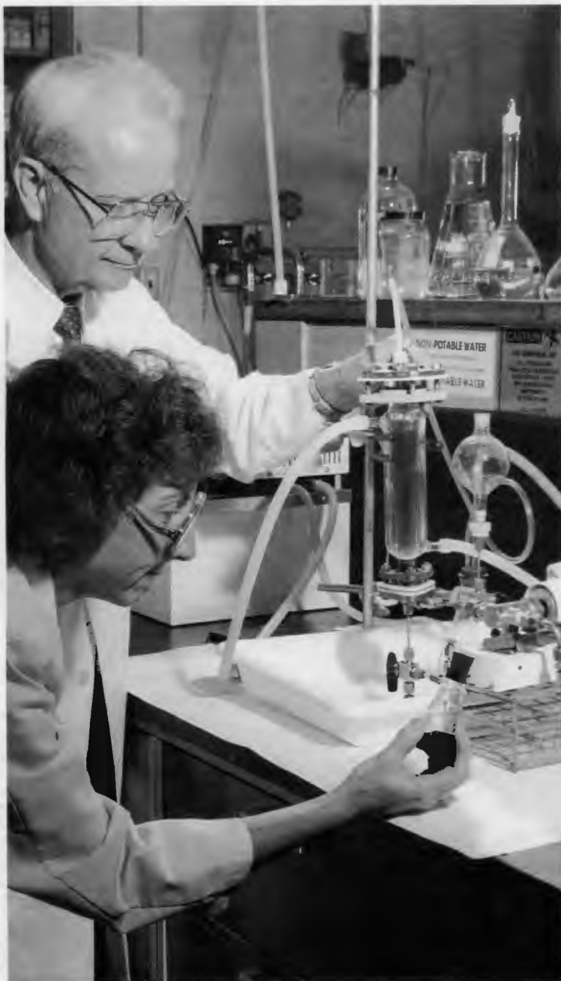
Chuck Scott observes a fluidized-bed bioreactor in which solid coal is being converted to liquid fuel. Charlene Woodward holds a flask containing a sample of the product, which resulted from the use of bacterial enzymes as biocatalysts for the conversion process.
