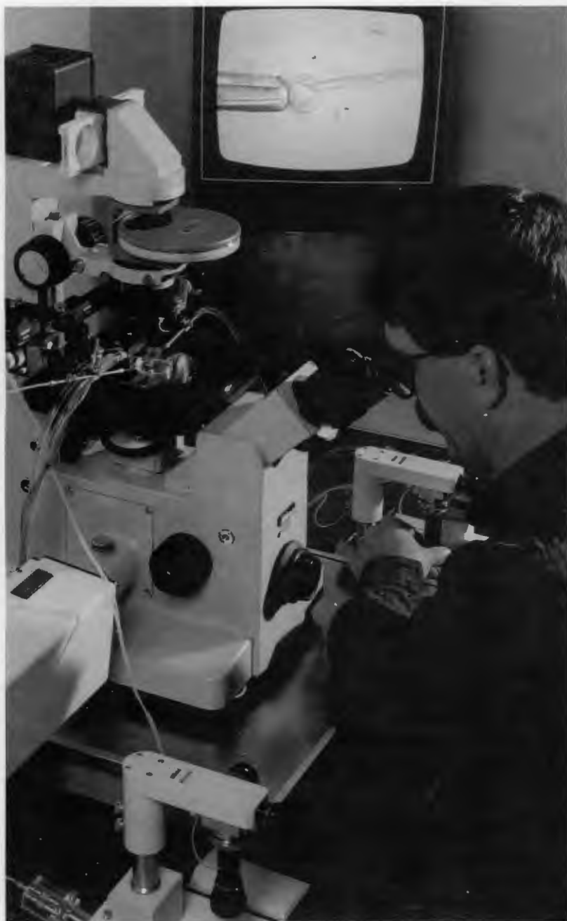
Through a microscope Mike Mucenski views objects that are displayed on the screen. The large strawlike tube (left) shown on the screen uses suction to hold a mouse embryo in place as embryonic stem cells (resembling tiny bubbles) from a different mouse are injected through the slender needle at right. Combining foreign cells with normal cells helps scientists determine the genes responsible for specific functions or diseases.
