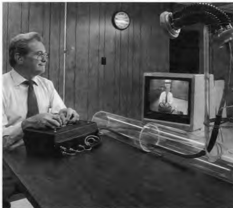
Don Box watches the Inchworm robot he developed creep through a pipe.—Photo by Bill Norris
