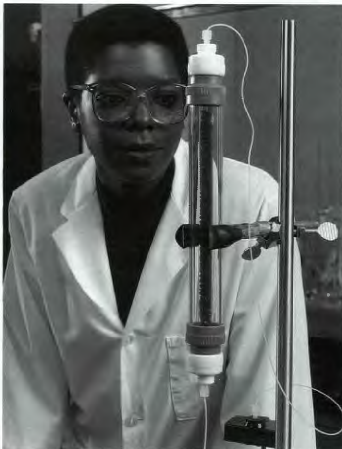
Brendlyn Faison examines gel beads immobilizing bacteria in a bioreactor for removing toxic metals from waste streams.
