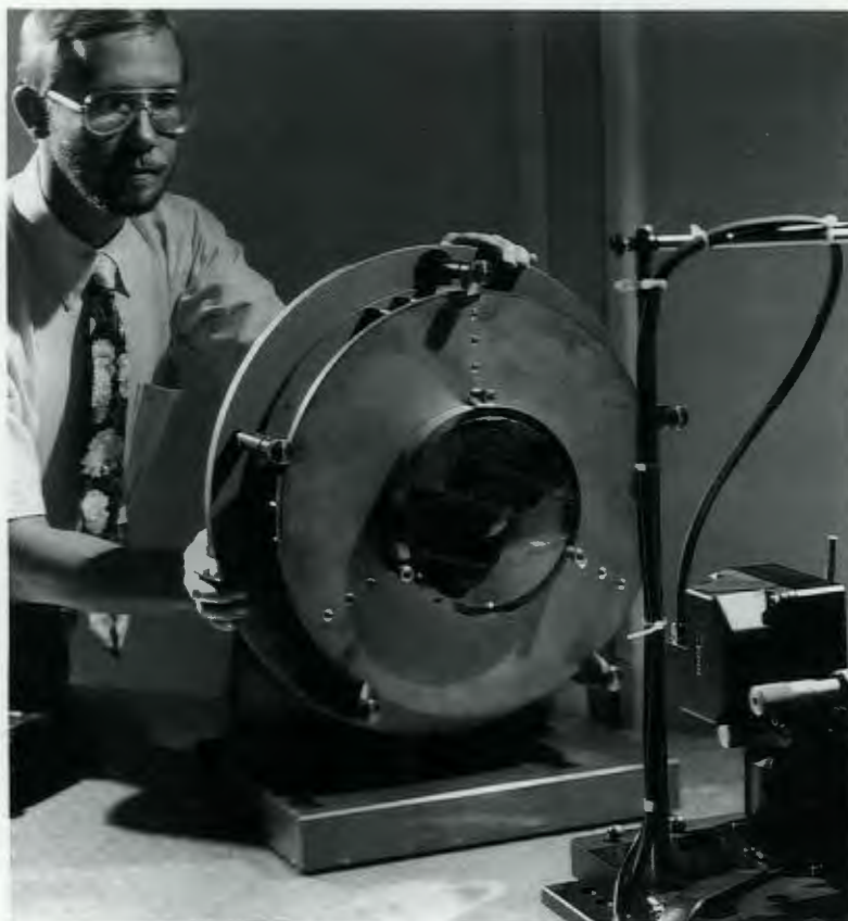
Curt Maxey operates a scanning Hartman device that uses laser light to confirm the shape of diamond-turned optical components to better than one-eighth wavelength. This is one of several advanced devices installed in the Optics MODIL established at ORNL to help the U.S. optics industry.
