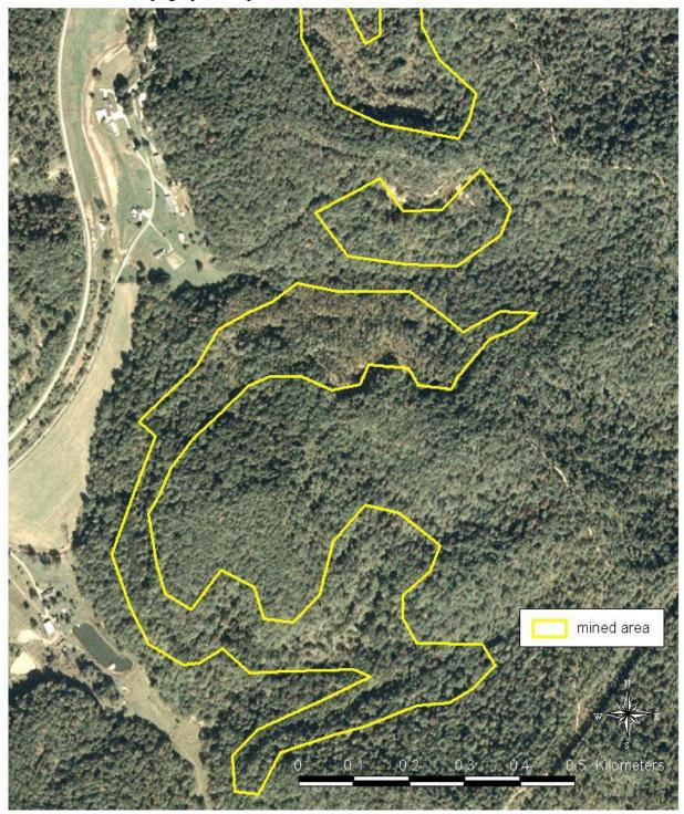
Figure 21B. Most active and abandoned or reclaimed surface mines and related ground disturbances can be detected on 2004 NAIP imagery, as in this example from eastern Muhlenberg County.
