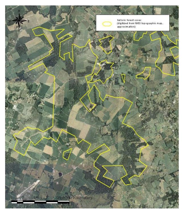
Figure 21. Even though recent or ongoing mining activities are often visible on aerial photos, surface scars and alterations caused by mining can be obstructed by maturing forest, as in this example of a 2004 NAIP image in Carter County where mined areas where revealed on topographic maps.
