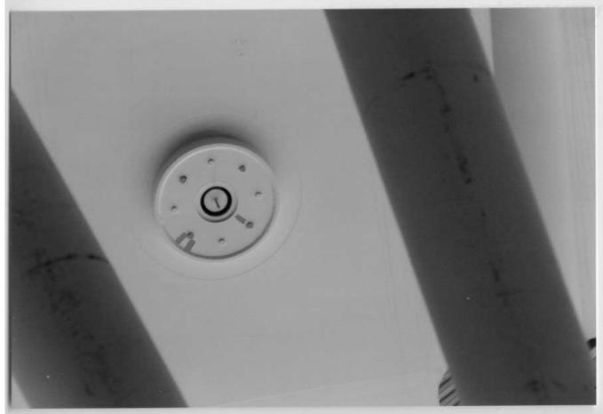
*Fig. 2: Location of target mark within cross-bar. The little sphere is mounted at the end of the rod in the middle of the circular plate.*
