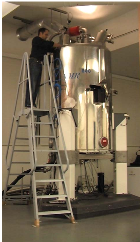
At Left: The 800MHz (18.8 Tesla) Varian NMR Spectrometer. Samples are loaded from the top, with the aid of a stepladder.
