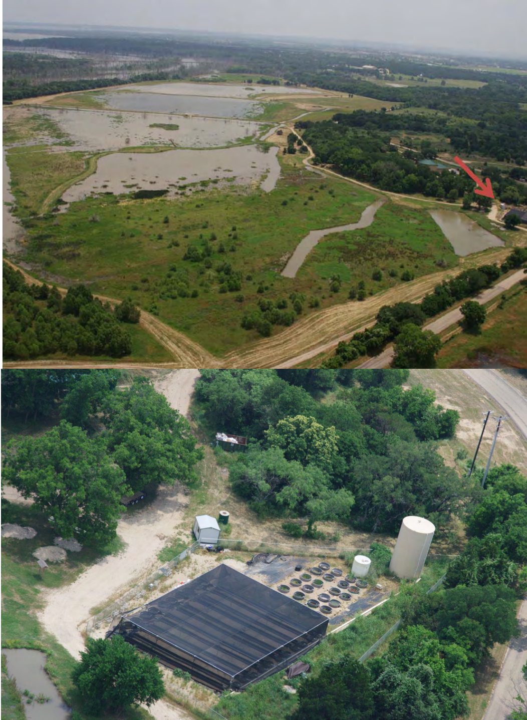
Figure 32. Aerial view of the Lake Waco Wetland and the location of the Baylor Experimental Aquatic Research (BEAR) stream facility (red arrow, upper panel). The lower panel is an aerial view the BEAR experimental stream facility (80' x 100', covered in 60% shade cloth), adjacent pond mesocosms, and a 40K gallon water tower used to store water pumped from the Lake Waco Wetlands en route to the experimental streams. See http://www.baylor.edu/aquaticlab/index.php?id=45868 for a video tour of the BEAR streams.
