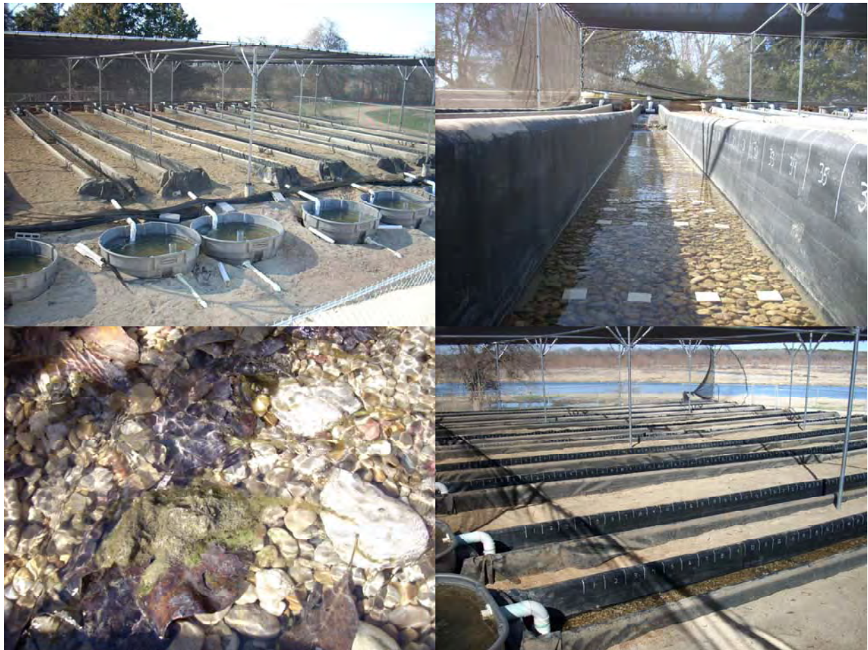
Figure 33. Collage of BEAR stream photographs illustrating the layout of the stream facility (top left), a view from within a glide section of a stream channel (top right), the substrate of a typical riffle section during the colonization phase of the study (bottom left), and a lateral view of the streams from the far left side of the facility, looking toward the adjacent Lake Waco Wetlands.
