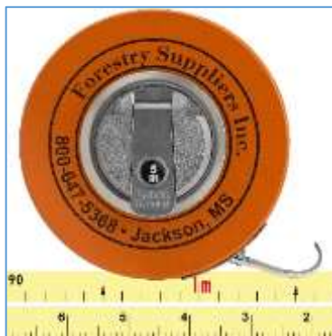
Figure 6. A commonly used dbh tape, which can be used as a meter tape and diameter tape.
