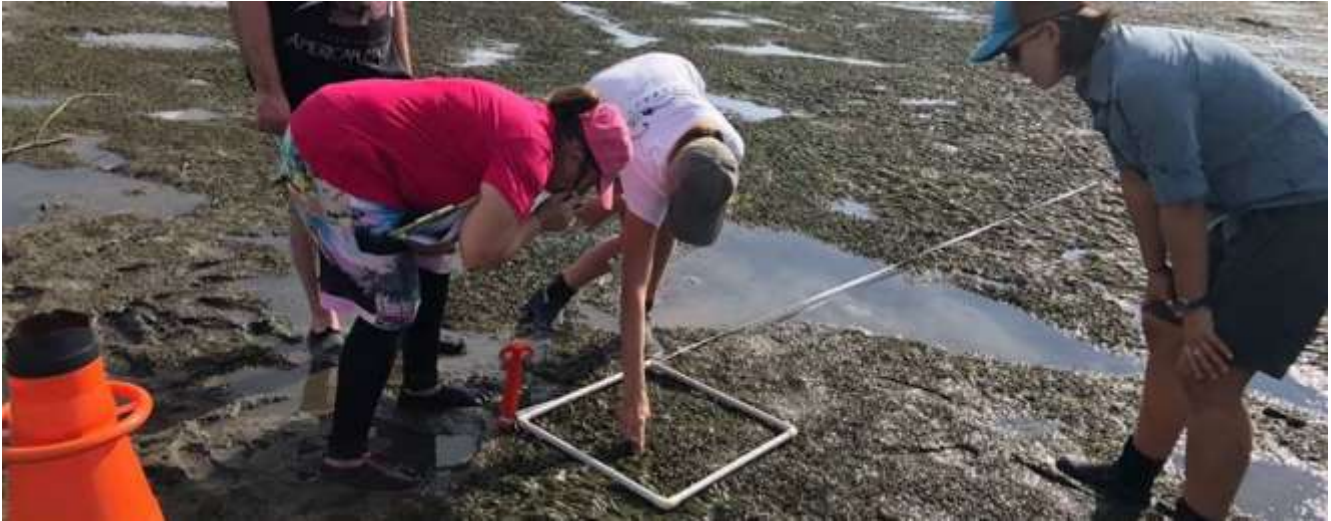
Figure 24. A seagrass bed survey along the Gold Coast, Australia. The quadrat in use is made from cheap PVC materials and is easy to transport. Source: SeagrassWatch (2021)
