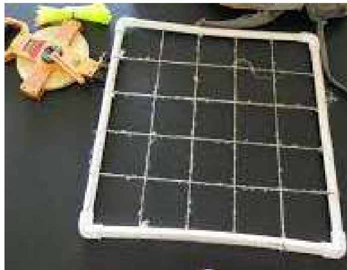
Figure 25. Plastic PVC piping quadrat with grid cells. Source: SeagrassWatch (2021)
