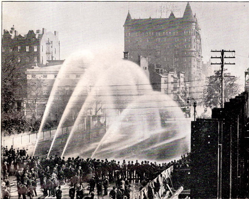
OFFICIAL TEST OF HIGH-PRESSURE WATER MAINS TRAVERSING THE PHILADELPHIA "FIRE BELT." The upper of these two pictures was made with Series VII a, No. 17, with 12 inch focus. The lower picture was made with the rear combination of the same lens.
