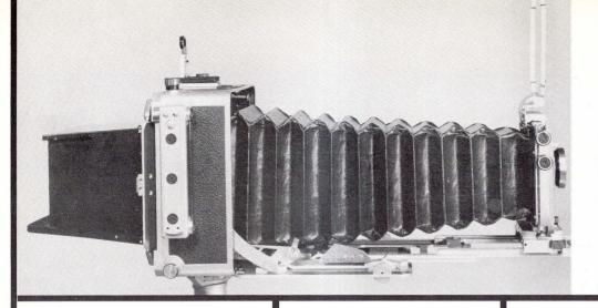
Triple extension bellows. Hand made from selected soft leather. Extends to 17 inches. Operated by large focusing knobs on both sides of camera. Obtains extreme closeups. Permits 1:1 copying.
