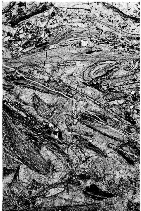
Fig. 3. Limestone (bivalve biosparudite) of the Tachigaya formation at the southern bank of Kitaosoki river, Tachigaya ( \times 10 ). Numerous bivalvian shell fragments cemented by sparry calcite.
