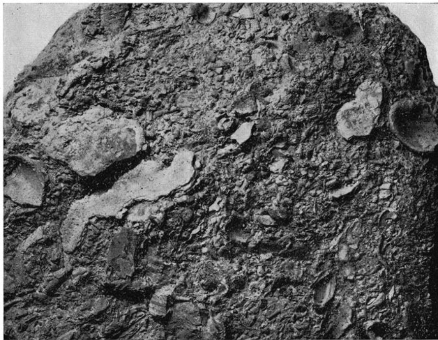
Fig. 43. Shell fragment limestone with lamellibranchs, brachiopods, bryozoans, echinoderms, corals, a. o. Senonian. Balsberg, Scania. (Pl. 645.) — 1/1.
