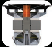
Two-part low-profile "i-beam" cone construction. 1/2" split voice coil construction. Oppositely wound turns on coils eliminate motor non-linearity.
