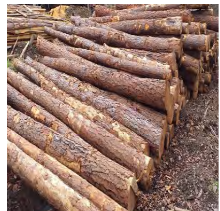
Figure 9: Log yards not in good condition and logs piled on the ground without proper bearers. This was one of the most common practice by most sawmills in Fiji. A well maintained yard with proper bearers will protect logs from blue stain and other defects and reduce sawmill losses.
