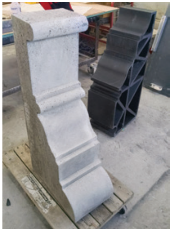
This insert (4) was cast by Thermawood for Gate Precast during a test of 3-D printed forms. The piece was set into a larger form to create the intricate face of a 1-ft-wide cornice, to see if it could replicate the actual 30-ft-long cornice installed on a Nordstrom store in New York, N.Y. Photo: Gate Precast.
