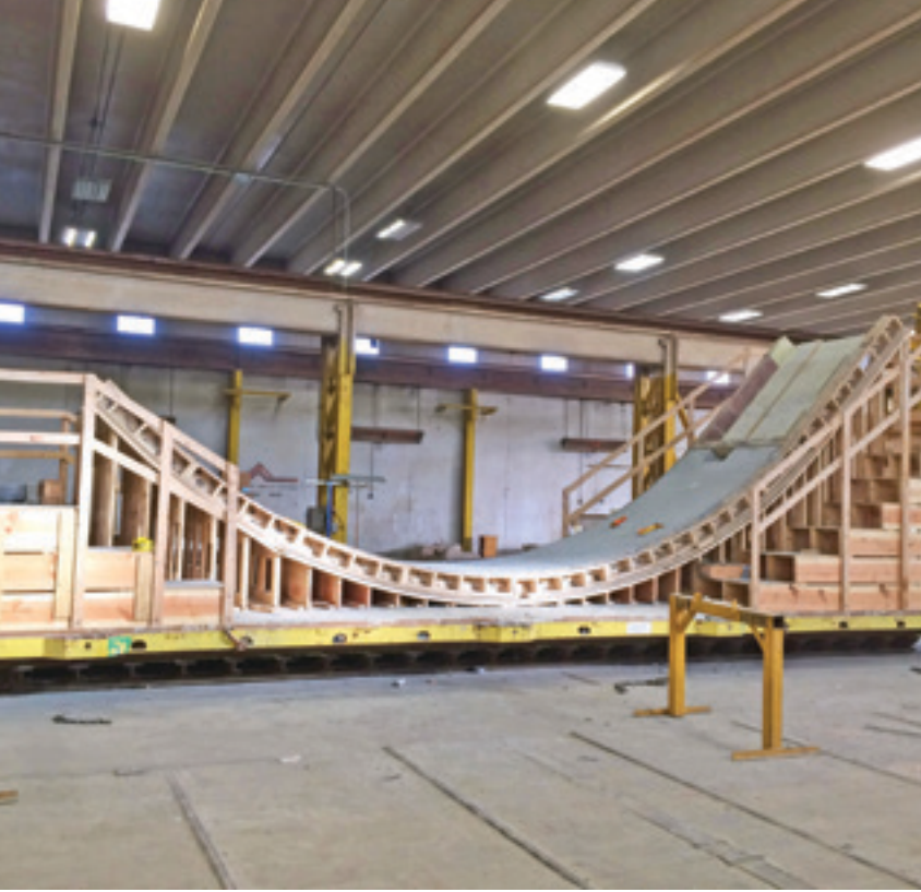
Rocky Mountain Prestress developed custom forms to cast more than 50 curved spandrel panels. Photo: Rocky Mountain Prestress.
