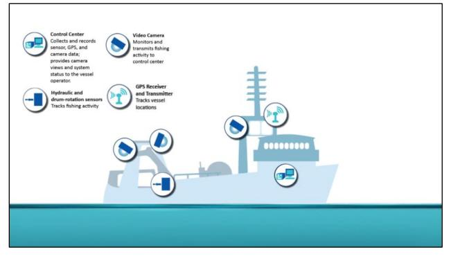
Figure 4. Example EM system and components onboard a trawl vessel.
