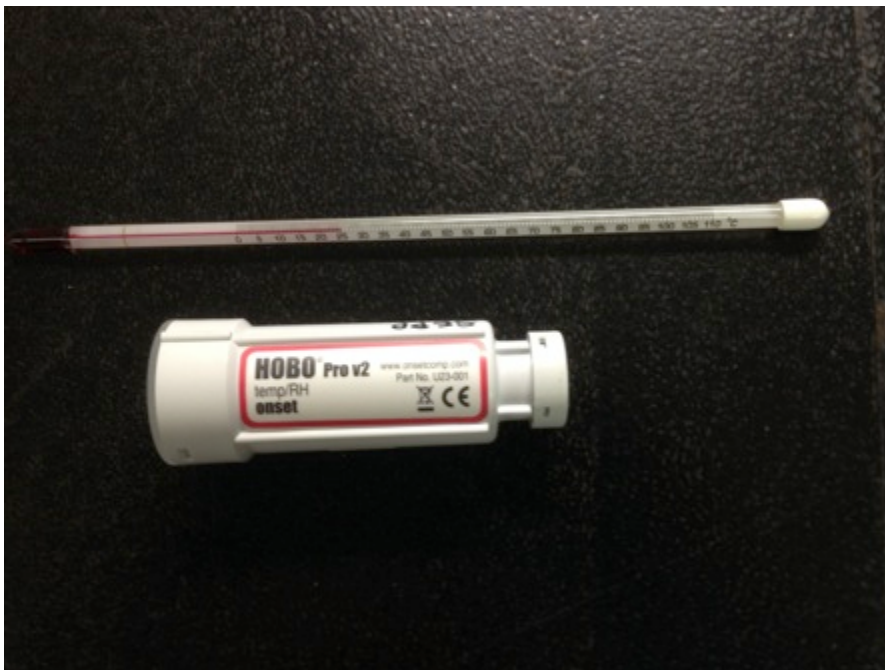
Figure A. Electronic and analog means to monitor temperatures in environmental chambers.
