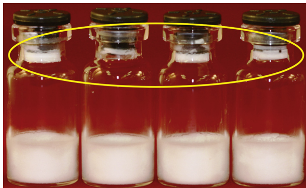
Figure 4. Product ejection: usually results in dried product being deposited in the stopper region of the vial.
